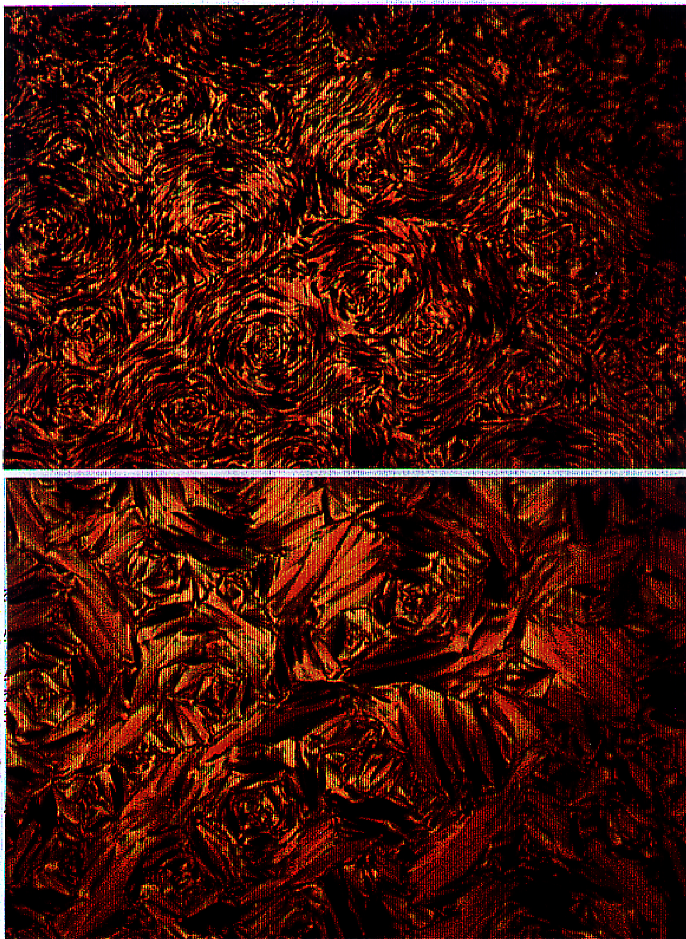
Fig. 3.24 Polarizing optical micrographs of M10 Filament texture of TGB A and spiral texture of S A phase at 129 °C (upper); "Rose" texture of S A phase at 129 °C (lower).
