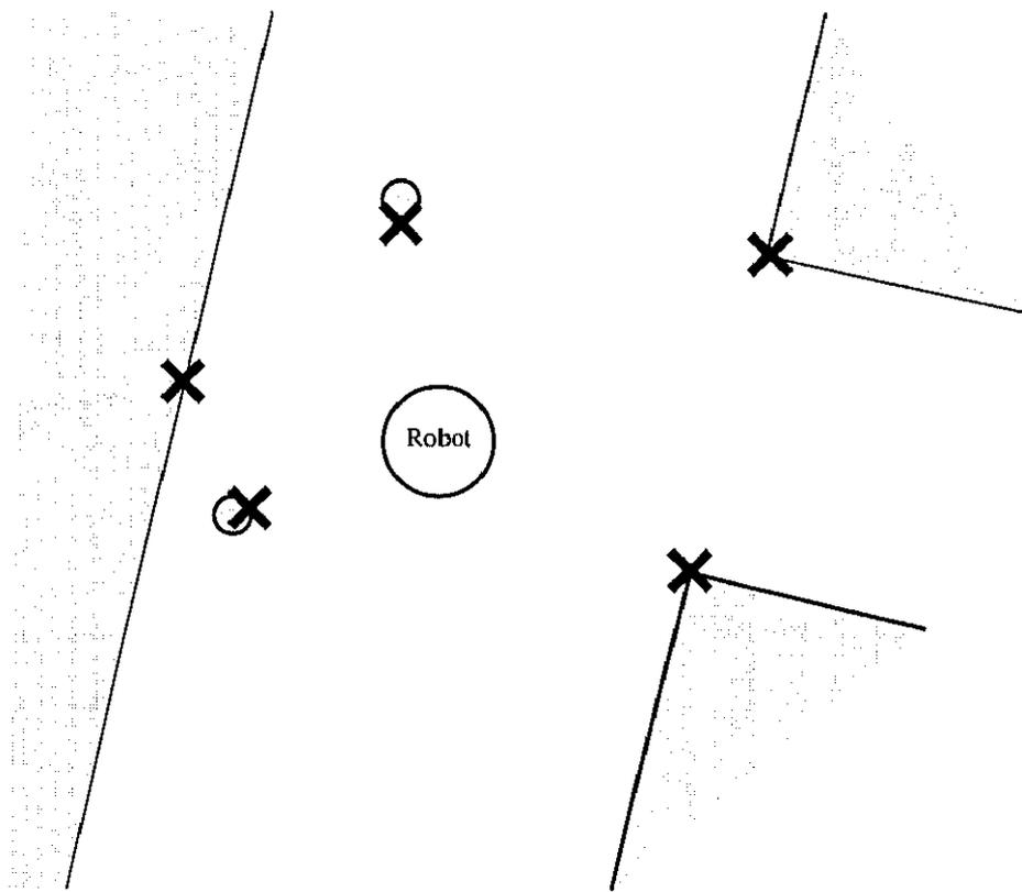
Figure 1.8: Examples of reflecting points in environment.
