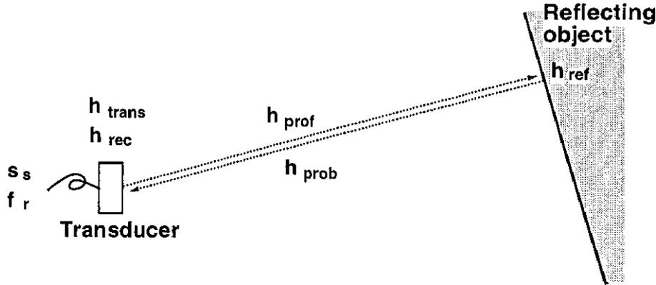
Figure 1.5: Linear propagation model
