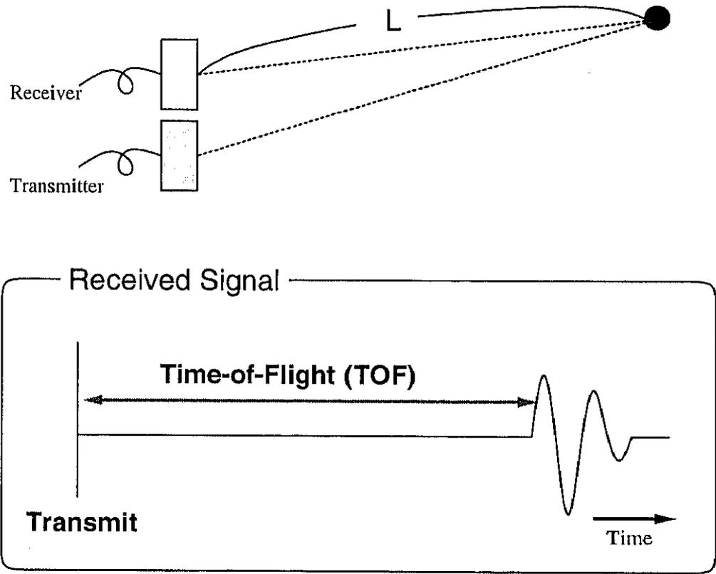
Figure 1.1: Pulse-echo method ultrasonic sensor.  $L$  is distance to the object,  $TOF$  is measured time interval between transmit and receive.
