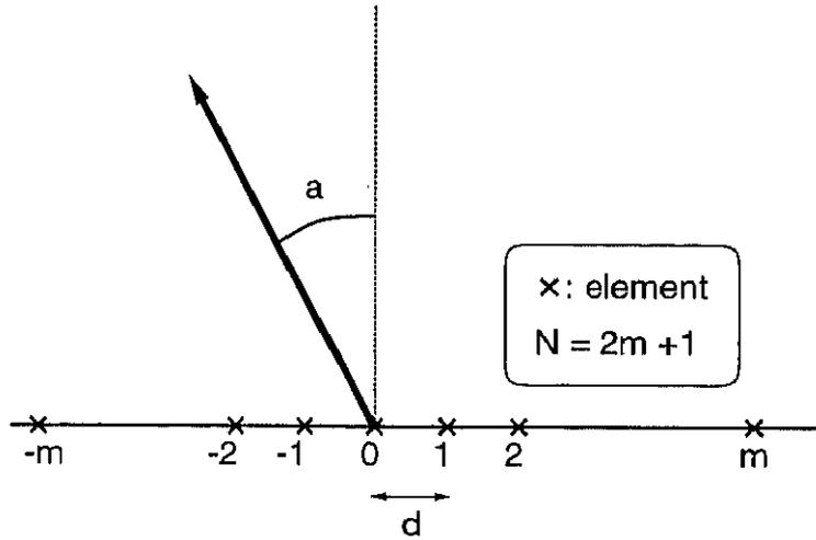
Figure 1.3: Electronic beam scanning method.  $N$  pieces of elements are aligned at distance  $d$   $a$  is beam angle.
