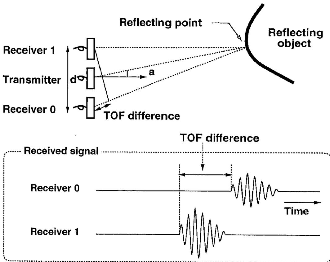
Figure 1.4: Accurate direction measurement by using TOF difference.
