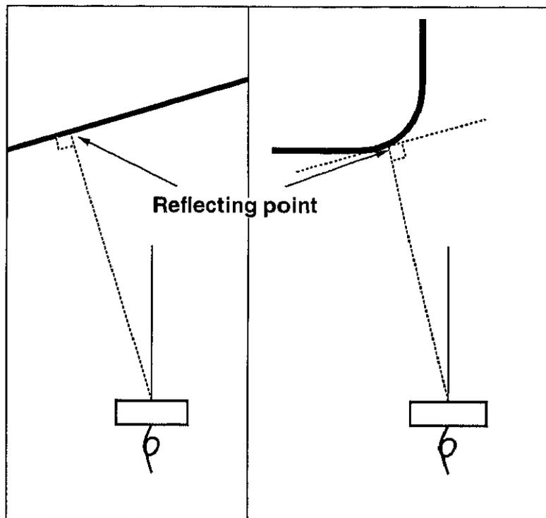
Figure 1.7: The bearing angle to the reflecting point is showing the perpendicular direction of the nearest point.
