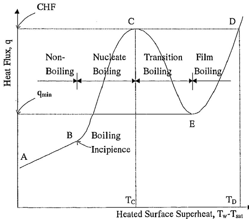
Fig1-1 Boiling Curve
