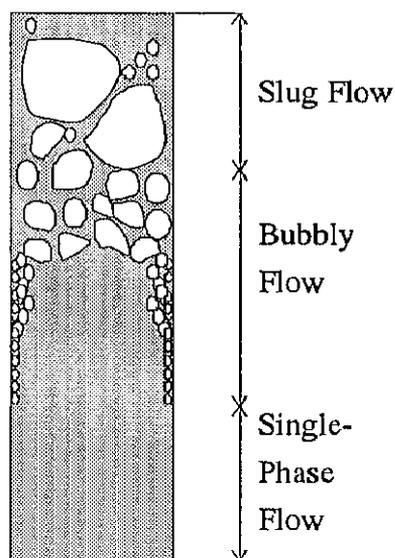
Fig.1-2: The First Kind of Flow Pattern of the Subcooled Flow Boiling
