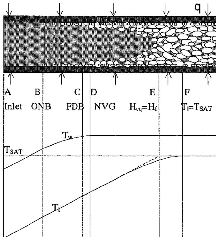
Figure 1-4 Schematic Representations of Flow Regimes and Wall Temperature Variation in Subcooled Flow Boiling
