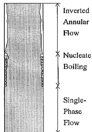
Fig.1-3: The Second Kind of Flow Pattern of the Subcooled Flow Boiling
