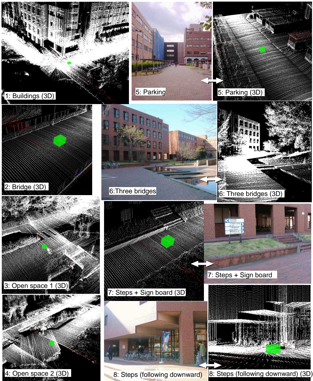
図 4.12: Snapshots of constructed walkway environment 3D structure
