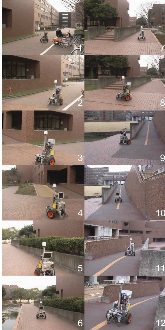
図 3.12: Snapshots of autonomous outdoor navigation using DGPS and odometry
