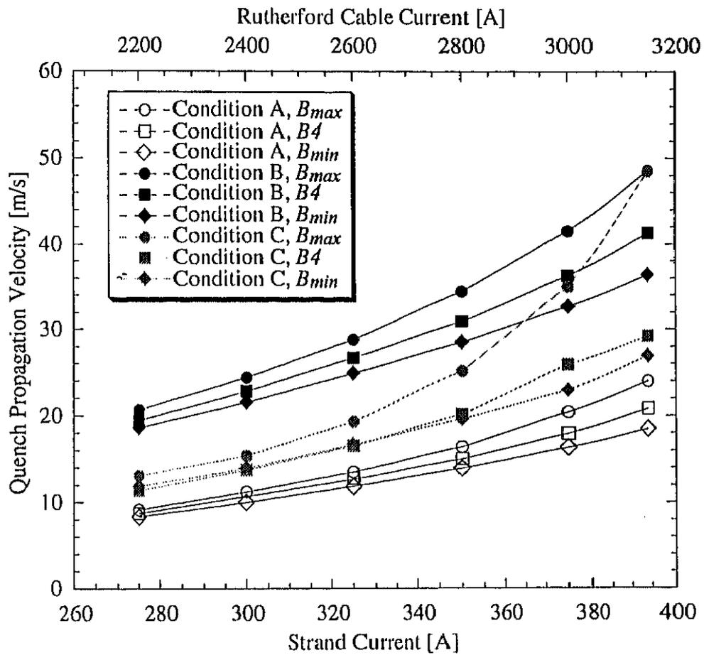
Fig. 3.3: Quench propagation velocities of a single strand measured under three cooling conditions as a function of strand current.
