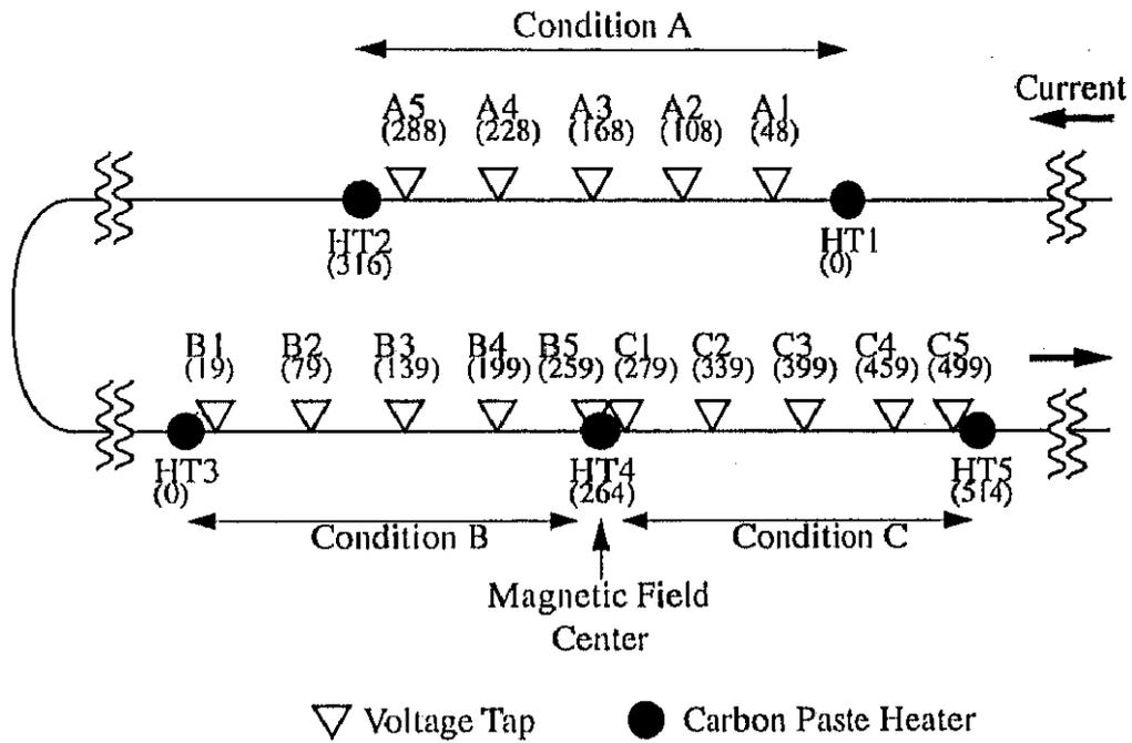
Fig. 3.2: Arrangement of three cooling conditions and positions of the voltage taps and the heaters. Condition A is the strand without thermal insulation, condition B is the strand covered with epoxy for thermal insulation, and condition C is the strand wrapped by polyimide tape with 50% overlap. The numbers in parentheses are the relative distances from heater HT1 or HT3.
