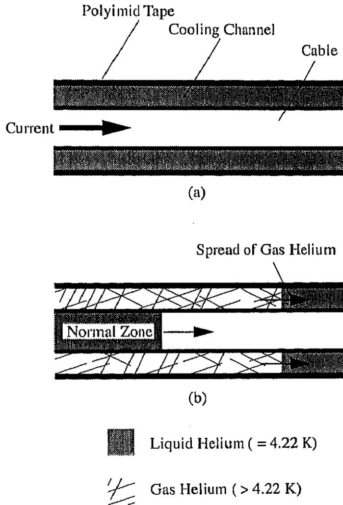
Fig. 3.6: Illustration of helium in a cooling channel around the cable. (a): before quench, (b): during quench propagation.
