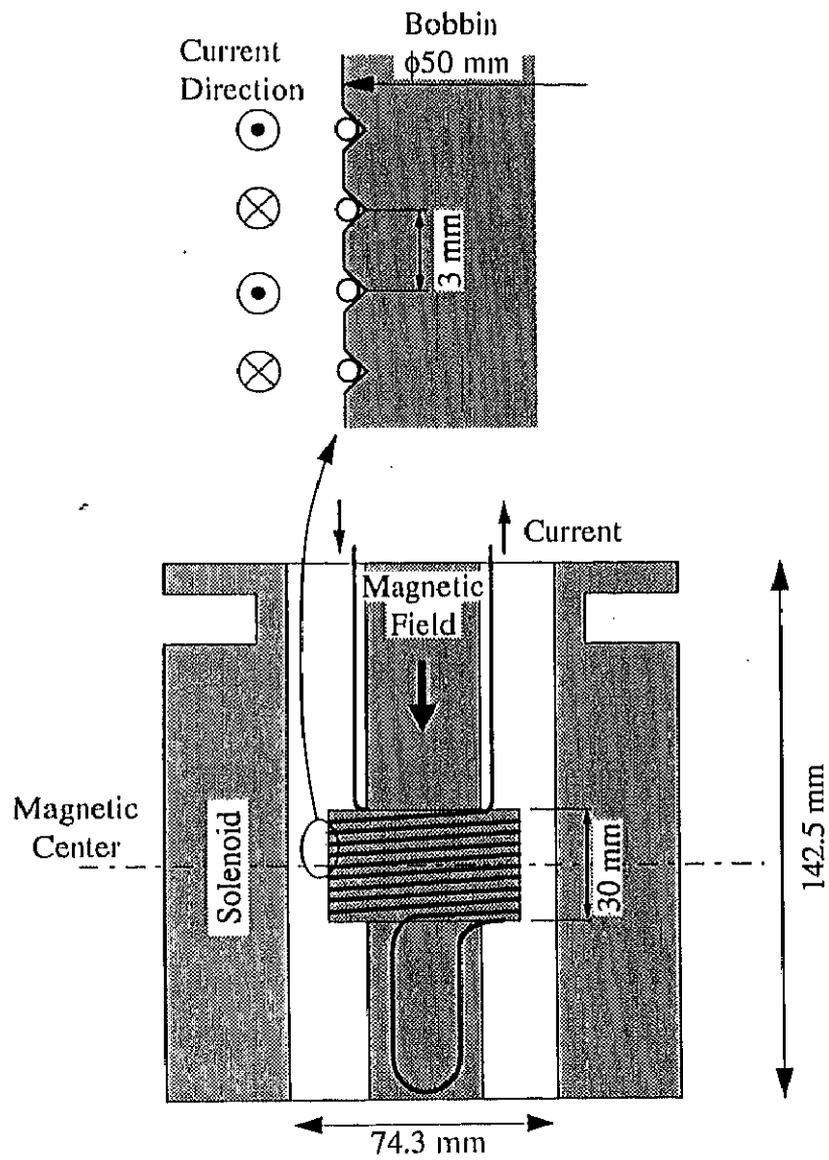
Fig. 3.1: Overview of the experimental setup for the single strand tests.
