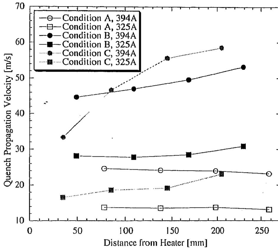
Fig. 3.4: Quench propagation velocities as a function of distance from the heater to the center of voltage tap couple at  $B_{max}$ .
