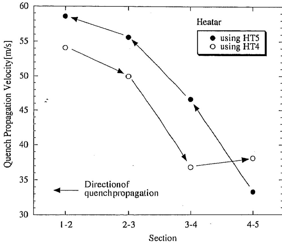
Fig. 3.5: Quench propagation velocities on every pair of voltage taps in condition C at the strand current of 394 A at  $B_{max}$ .
