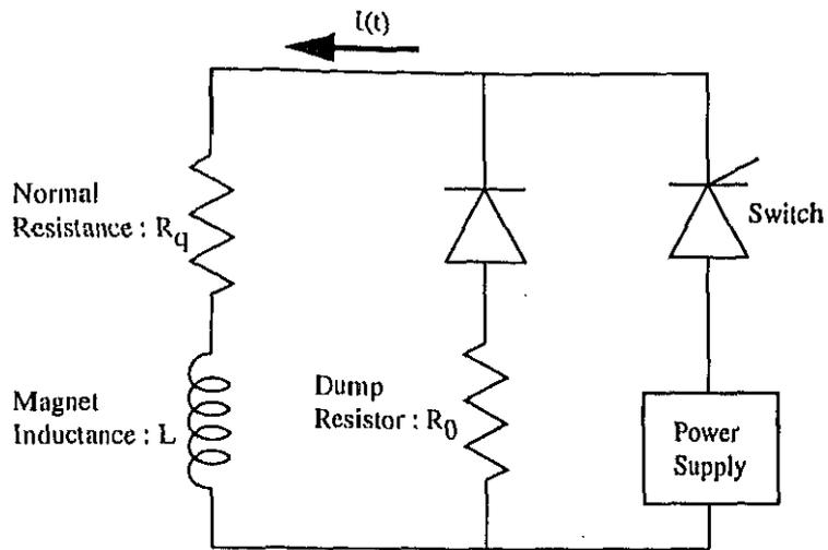
Fig. 1.3: Simple protection circuit with an external dump resistor.
