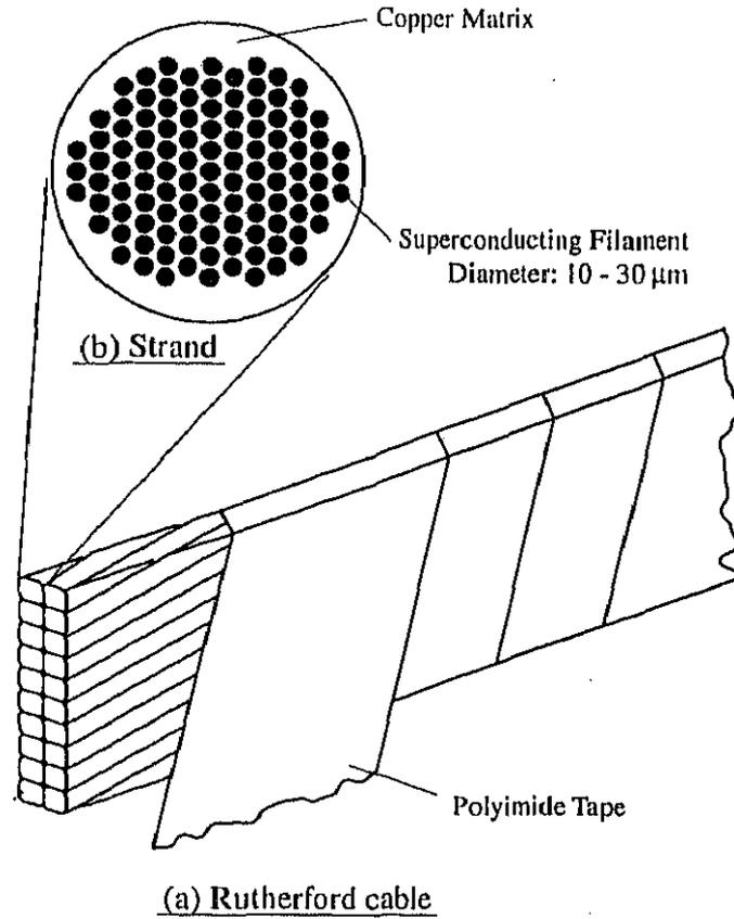
Fig. 1.1: Schematic view of a Rutherford cable and a strand cross section.
