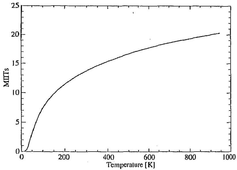
Fig. 1.2: Example of MIITs calculation. The parameters are those of the outer cable parameters for LHC insertion quadrupole magnets.
