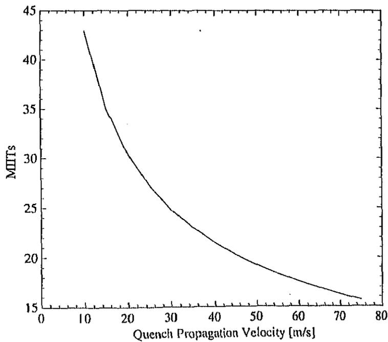
Fig. 1.4: Example of calculated MITs as a function of the quench propagation velocity.
