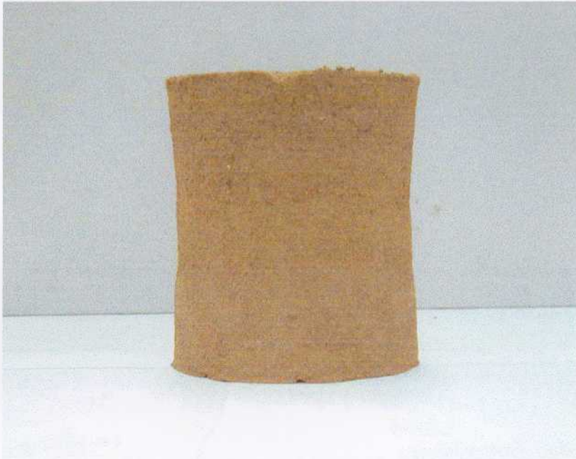
Fig. B-1 Soil specimen after tested and dried in oven.
