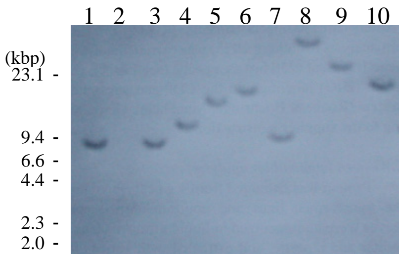
Fig. 22. Southern blot analysis of putative transformed plants. Genomic DNA digested with Eco RV and hybridized with the cryIAb specific probe.
