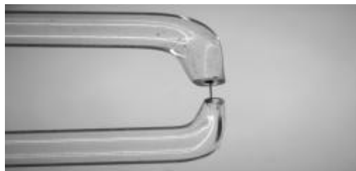
Fig. 4-2-3. Photograph showing a single antennal bridge between paired capillary glass electrodes.
