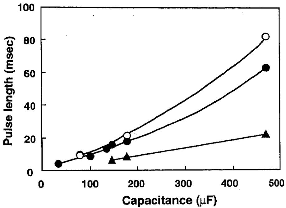
Fig. 3-4. Effect of buffer concentration on pulse length.
