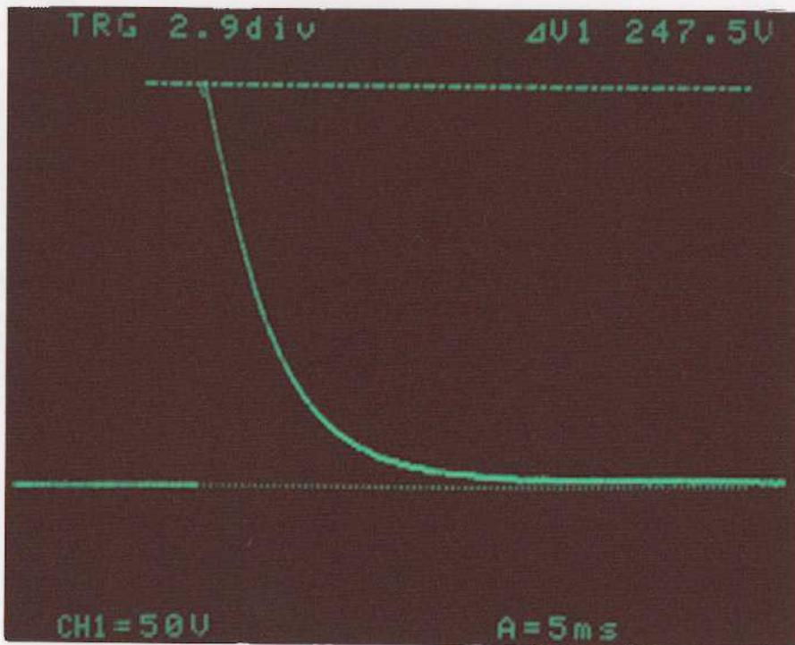
Fig. 3-3. The waveform of the electroporator.
