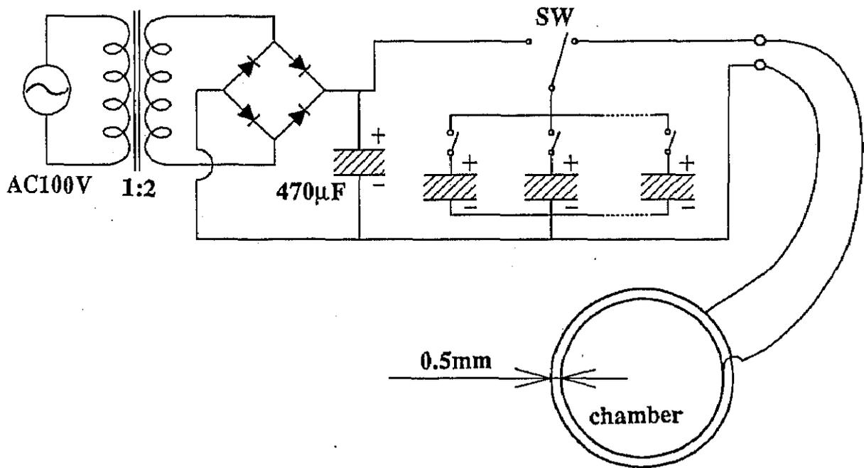
Fig. 3-2. Circuit diagram of the electroporator.
