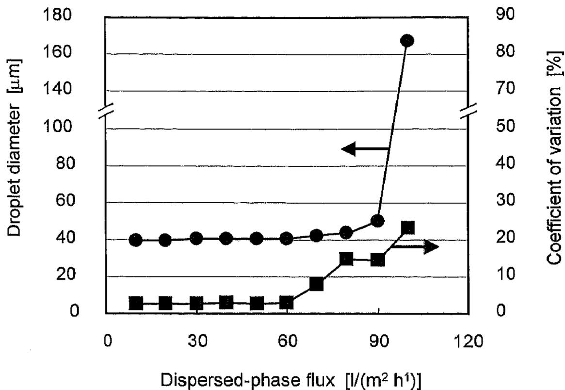
Fig. 6.1.5 Effect of dispersed phase flux on average diameter and coefficient of variation of droplets formed using TMC-B for soybean oil/1.0 wt.% SDS aqueous solution system. A dispersed phase flux of 60 l/(m² h) corresponds to a droplet formation volume rate of 6.0 ml/h per plate.
