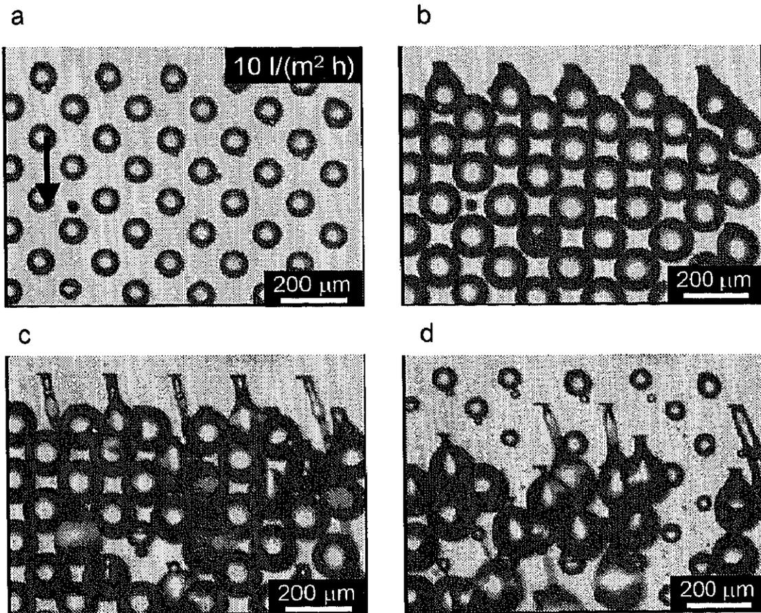
Fig. 6.2.3 Microscopic photographs of droplet formation from an oblong straight-through MC for soybean/(1.0 wt.% CTAB) water system. (a)-(d) Continuous phase flow-driven droplet formation.
