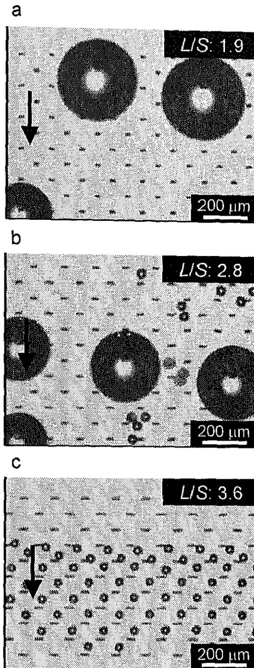
Fig. 6.1.3 Microscopic photographs of droplet formation from oblong straight-through MCs with different channel elongations for soybean oil / water (1.0 wt.% SDS) system. (a) Continuous droplet growth; (b) combination of spontaneous droplet formation and continuous droplet growth; (c) spontaneous droplet formation with uniform droplet diameter.
