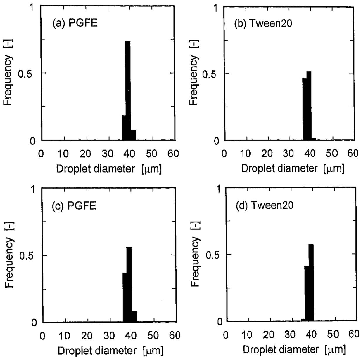
Fig. 6.3.4 Droplet diameter distribution for soybean oil-in-water emulsion droplets. (a), (b) O/W emulsion droplets just after formation; (c), (d) O/W emulsion droplets after recovery.
