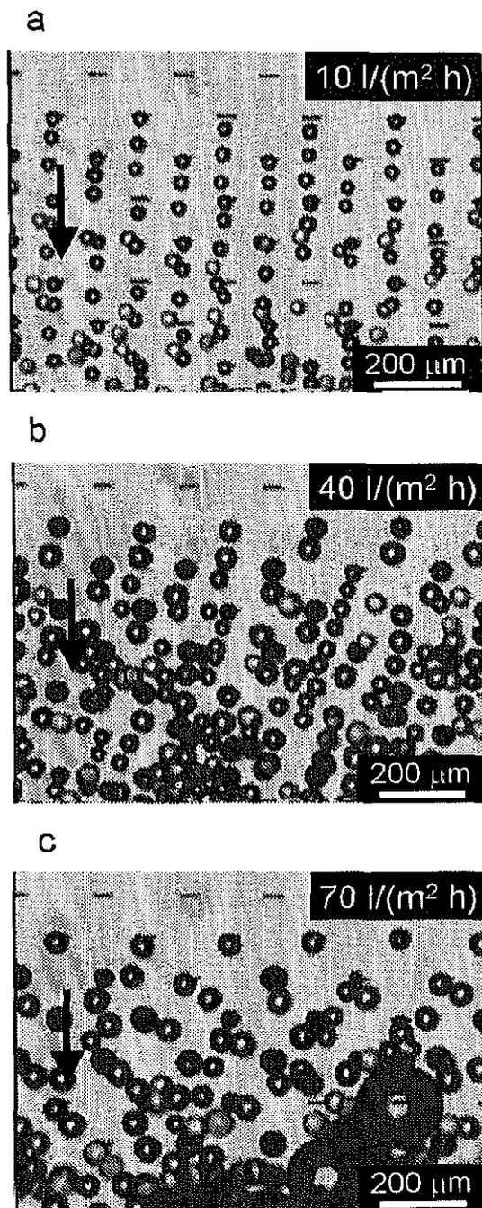
Fig. 6.2.1 Effect of dispersed phase flux for soybean oil/(1.0 wt.% Tween20) water system. (a) Size-stable zone; (b) size-expanding zone 1; (c) size-expanding zone 2. A dispersed phase flux of 40 l/(m<sup>2</sup> h) corresponds to a droplet formation volume rate of 4.0 ml/h per plate.
