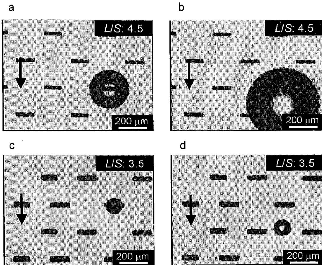
Fig. 6.1.6 Microscopic photographs of droplet formation from oblong straight-through MCs with smooth and distorted cross-sectional lines for soybean oil / water (1.0 wt.% SDS) system. (a), (b) Continuous phase flow-driven droplet formation from TMC-C5; (c), (d) spontaneous droplet formation from TMC-C'5.
