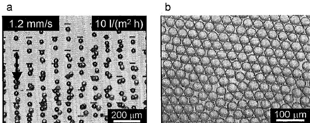
Fig. 6.3.3 Microscopic photographs of the straight-through MC emulsification process using TMC-2. (a), (b) Droplet formation and recovered monodisperse O/W emulsion droplets for a soybean oil/water (1.0 wt.% PGM) system.
