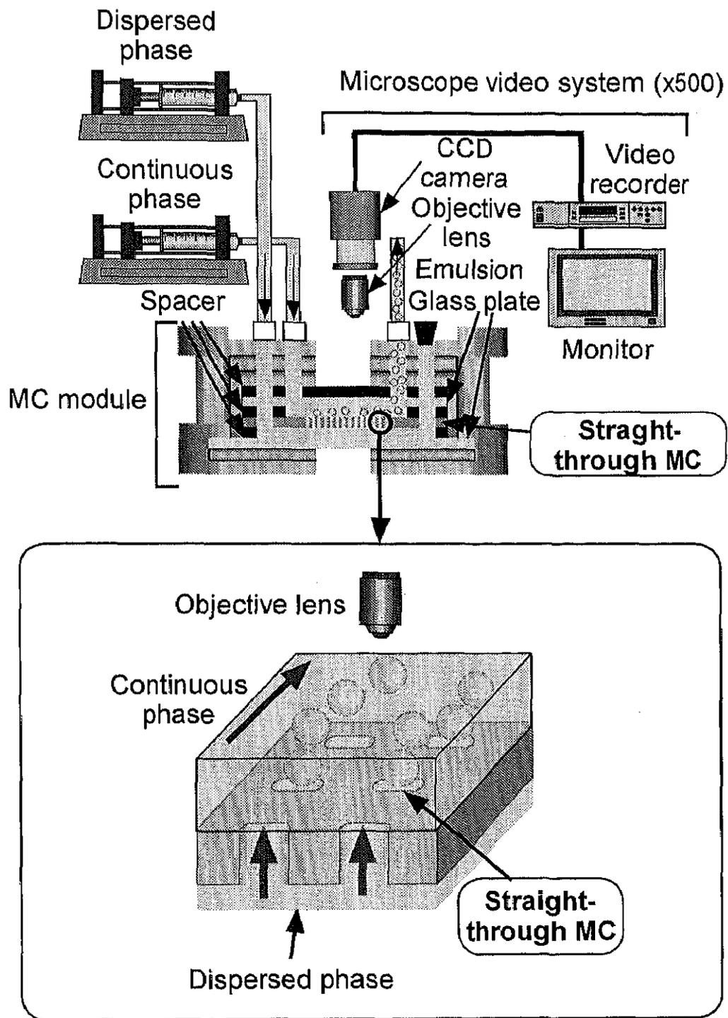
Fig. 6.1.2 Experimental setup and flow through the straight-through MC in the module.
