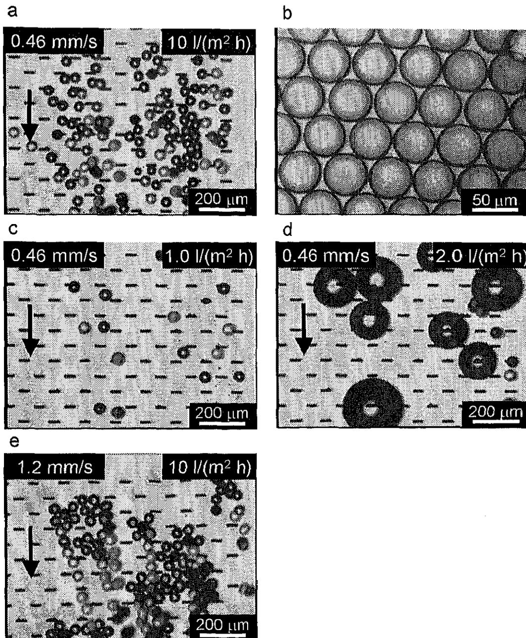
Fig. 6.3.1 Microscopic photographs of the straight-through MC emulsification process using TMC-1. (a), (b) Droplet formation and formed monodisperse O/W emulsion droplets for a soybean oil/water (1.0 wt.% PGM) system; (c), (d) droplet formation for a soybean oil/water (1.0 wt.% SE) system; (e) droplet formation for a soybean oil/water system. A dispersed phase flux of  $10 \text{ l}/(\text{m}^2 \text{ h})$  corresponds to a droplet formation volume rate of  $1.0 \text{ ml}/\text{h}$  per plate.
