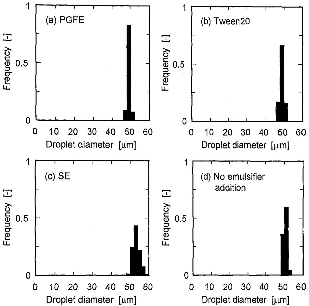
Fig. 6.3.2 Droplet diameter distribution for soybean oil-in-water emulsion droplets.
