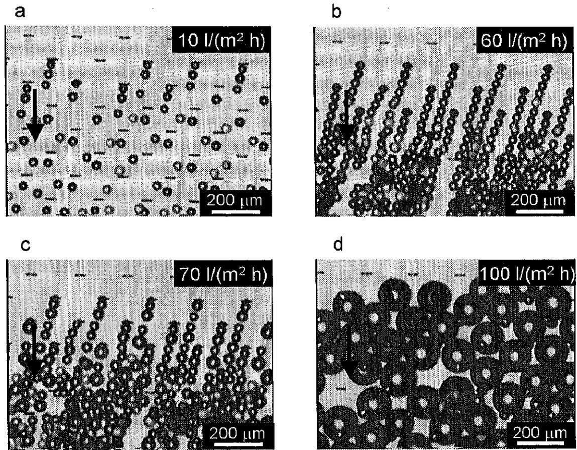
Fig. 6.1.4 Microscopic photographs of droplet formation from TMC2-1 for soybean oil / water (1.0 wt.% SDS) system. (a), (b) Size-stable zone; (c) size-expanding zone 1; (d) size-expanding zone 2. A dispersed phase flux of 60 l/(m<sup>2</sup> h) corresponds to a droplet formation volume rate of 6.0 ml/h per plate.
