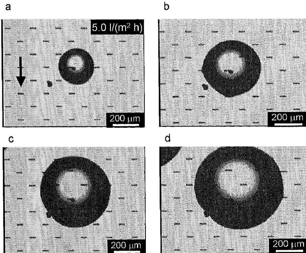
Fig. 6.2.4 Microscopic photographs of wetting of the dispersed oil phase on a channel surface for a soybean oil (2.0 wt.% TOMAC)/water system.
