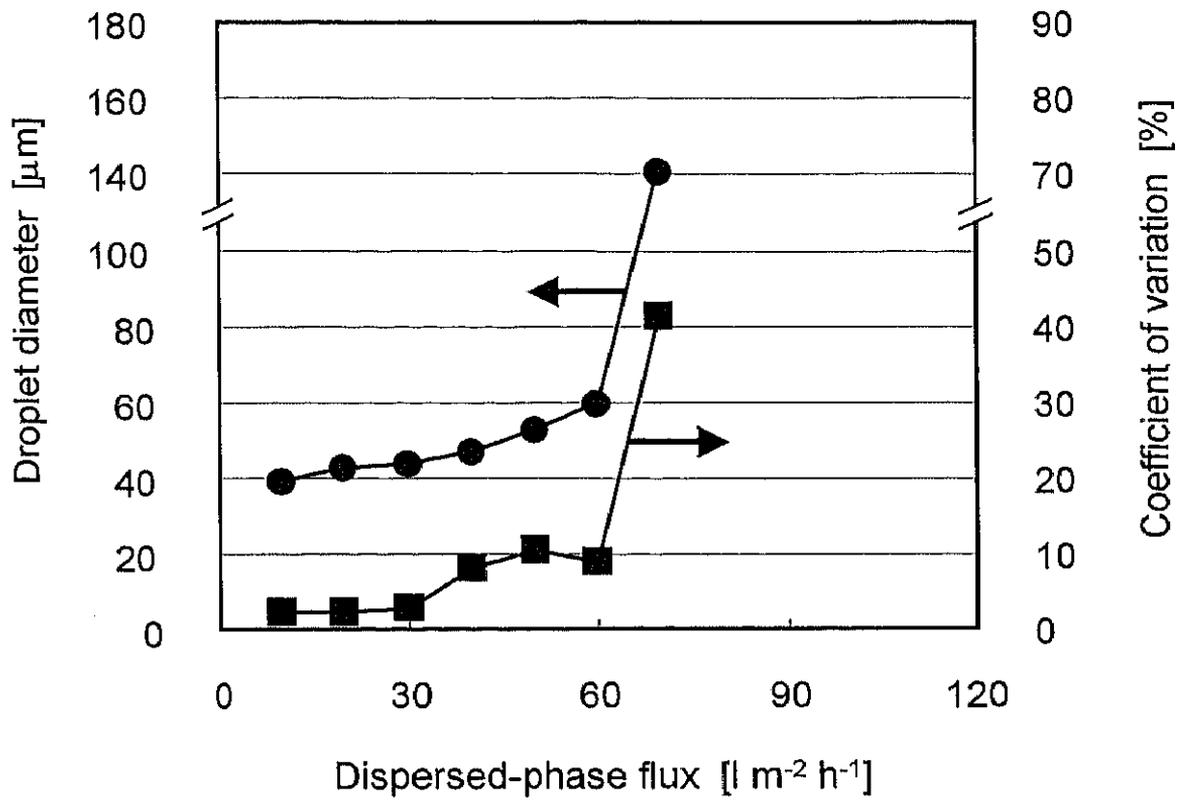
Fig. 6.2.2 Effect of dispersed phase flux on average diameter and coefficient of variation of droplets formed using TMC-B for soybean oil/1.0 wt.% Tween20 aqueous solution system. A dispersed phase flux of 30  $\text{l}/(\text{m}^2 \text{h})$  corresponds to a droplet formation volume rate of 3.0  $\text{ml}/\text{h}$  per plate.
