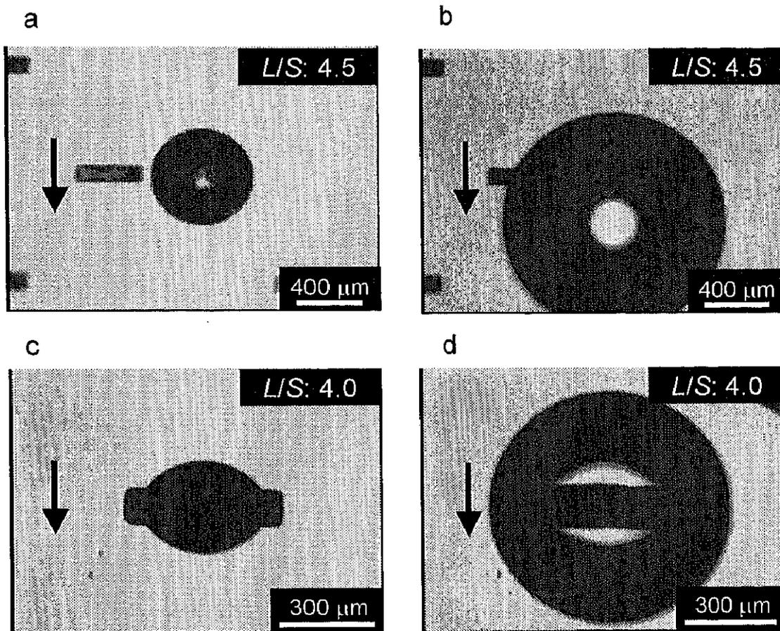
Fig. 6.1.7 Microscopic photographs of droplet formation from oblong straight-through MCs with smooth and distorted cross-sectional lines for soybean oil / water (1.0 wt.% SDS) system. (a), (b) Continuous phase flow-driven droplet formation from TMC-D5; (c), (d) continuous phase flow-driven droplet formation from TMC-D'5.
