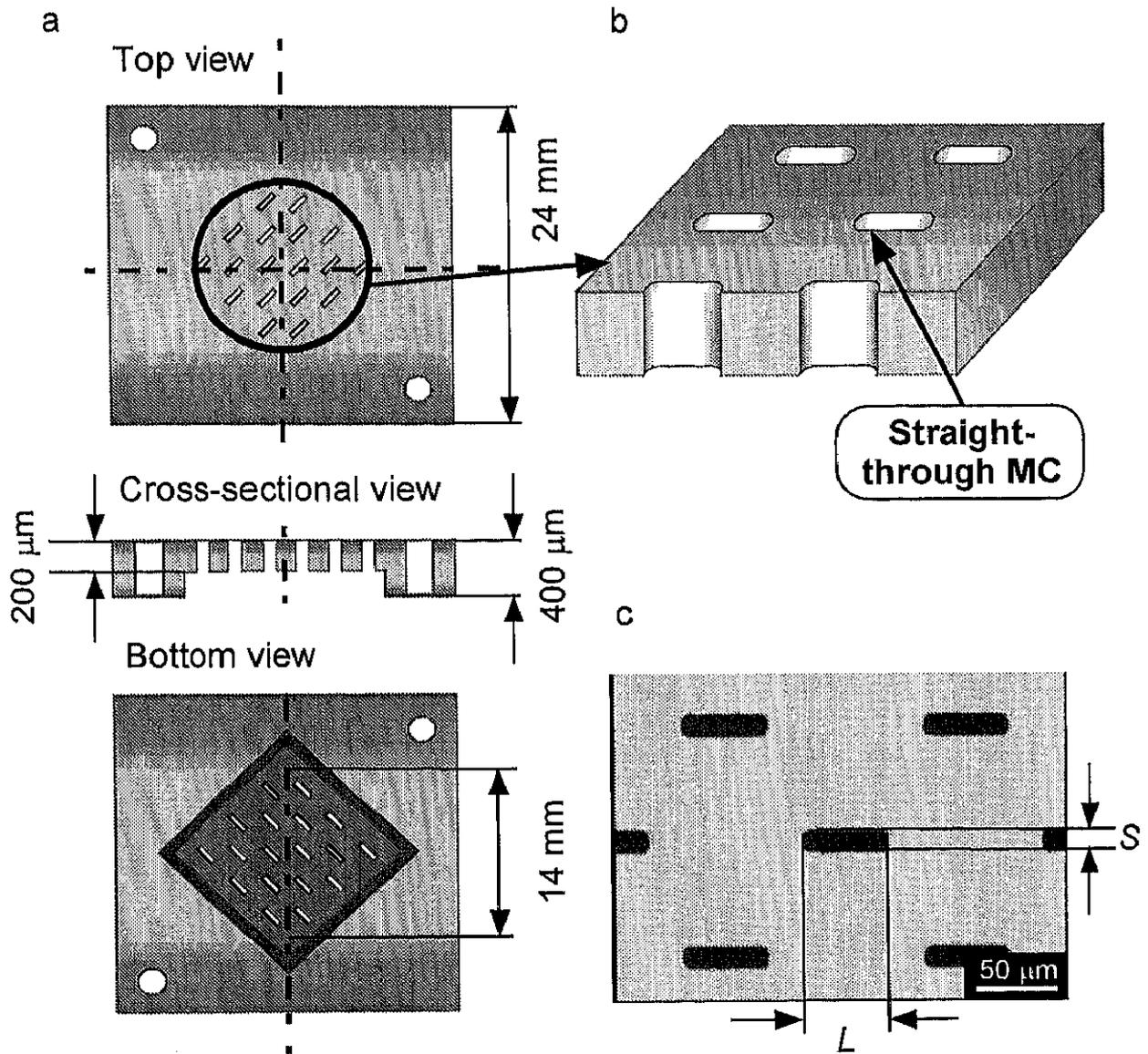
Fig. 6.1.1 Silicon straight-through MC plate. (a) Schematic drawing of the top view, and bottom view of the straight-through MC plate; (b) Schematic drawing of a straight-through MC; (c) a SEM photograph of an oblong straight-through MC.
