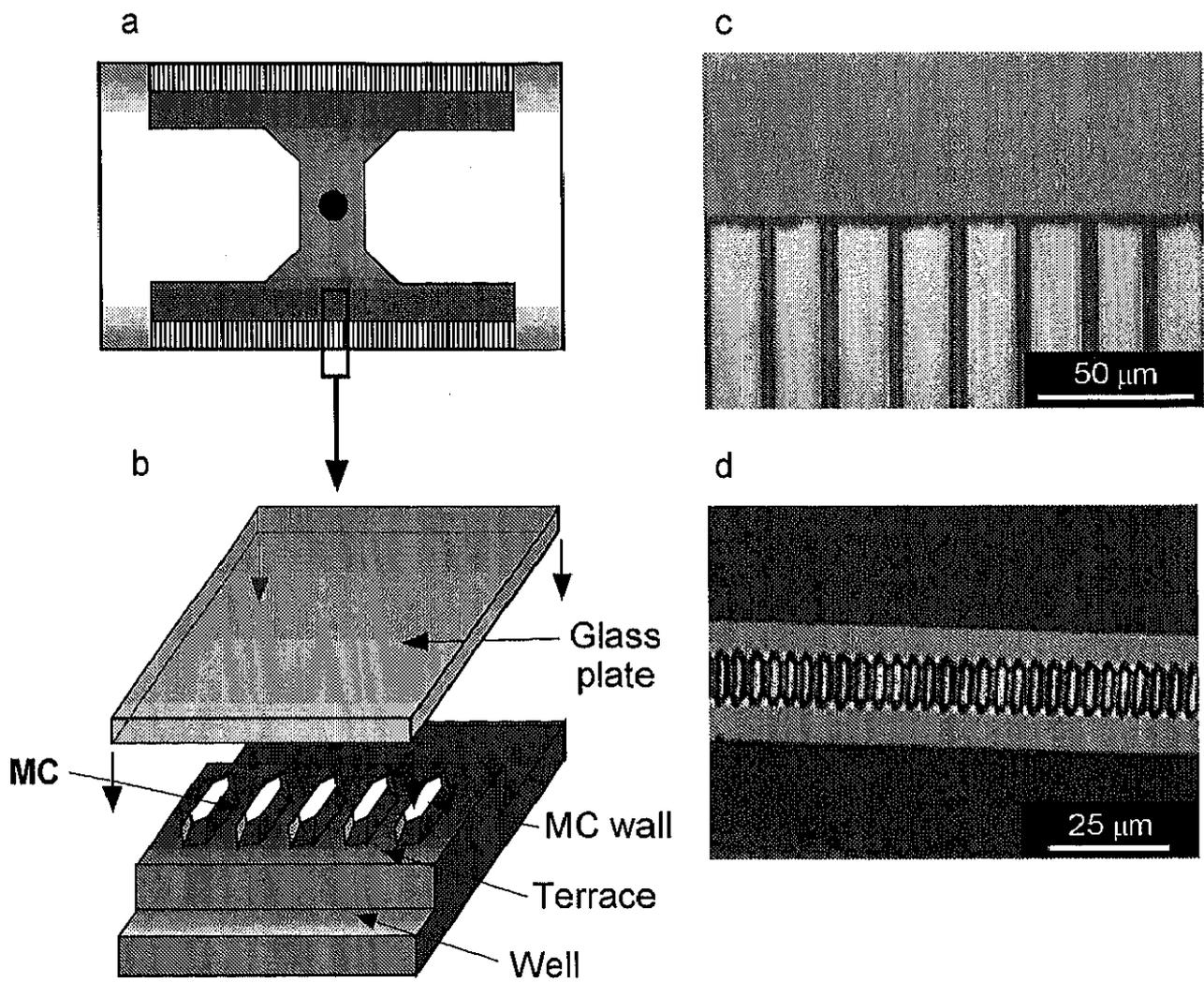
Fig. 2.1 Schematic diagram and photographs of silicon MC plate.
