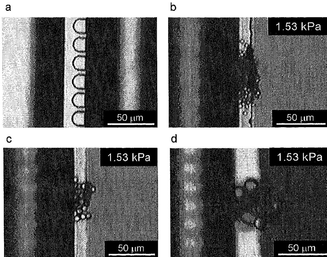
Fig. 2.4 Droplet formation using SMC-A4 ( $d_{eq} = 1.7 \mu\text{m}$ ). (a) Filled with continuous phase; (b)-(d) O/W emulsion droplets from different channels.
