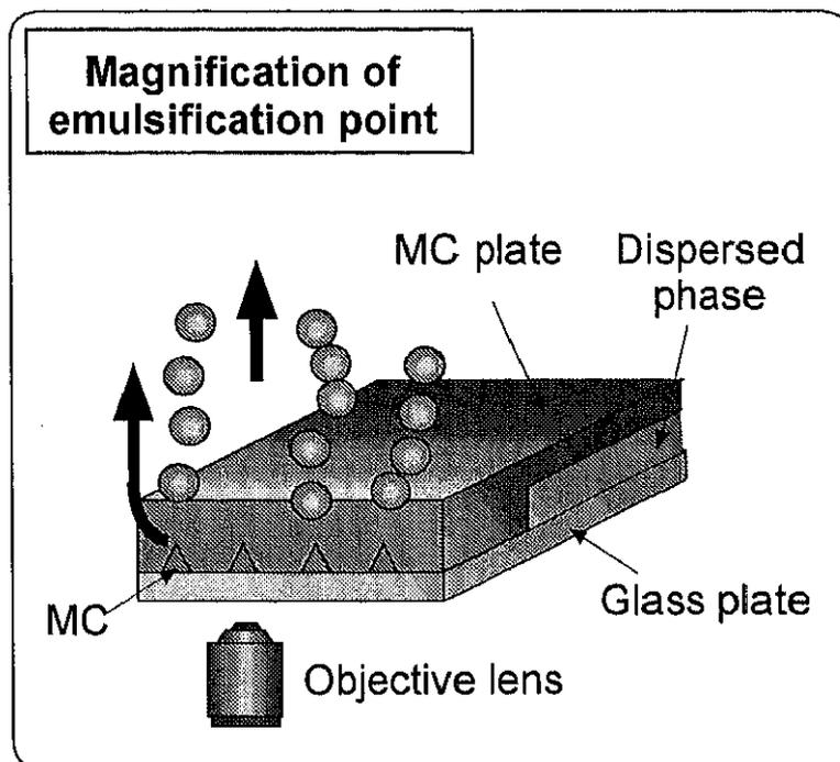
Fig. 2.2 Experimental setup for MC emulsification.
