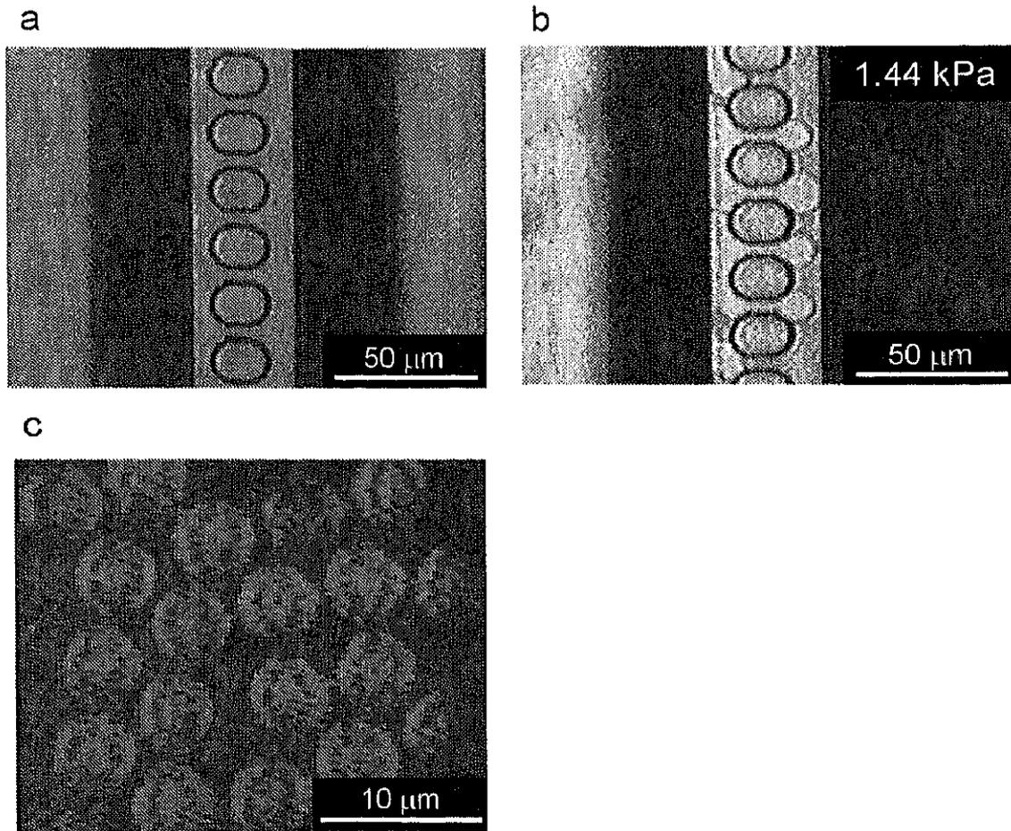
Fig. 2.5 Droplet formation using SMC-B4 ( $d_{\text{eq}} = 1.7 \mu\text{m}$ ). (a) Filled with continuous phase; (b) breaking through MC and droplet formation; (c) monodisperse O/W emulsion droplets.
