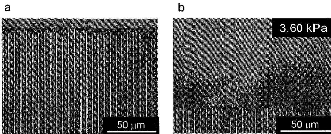
Fig. 2.3 Droplet formation using open-end MC ( $d_{eq}$  = MC equivalent diameter = 2.4  $\mu\text{m}$ ). (a) Filled with continuous phase; (b) breaking through MC and droplet formation.
