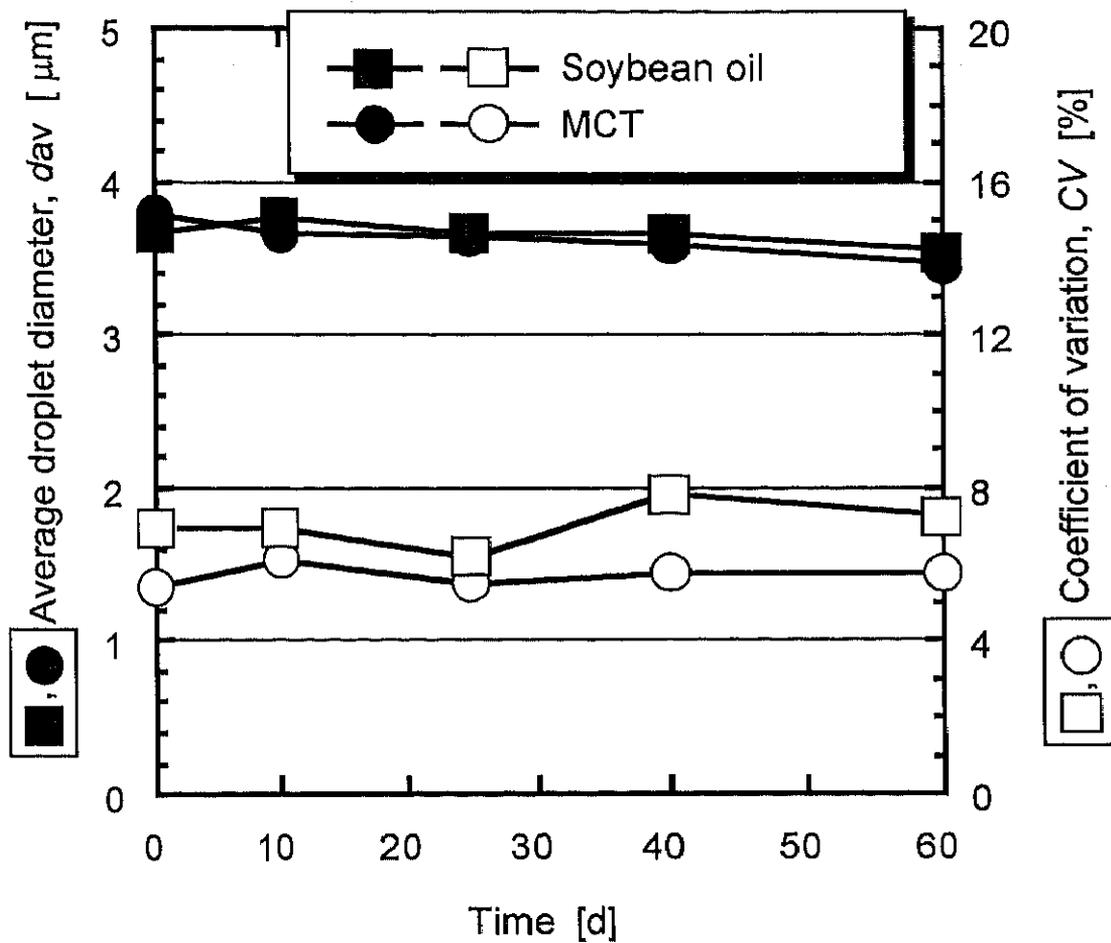
Fig. 2.6 Time course of the average droplet diameter and coefficient of variation of O/W emulsions recovered using SMC-B4 with pentaglycerol monolaurate as surfactant.
