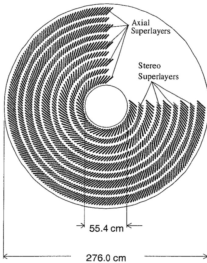
Figure 2.4: The CTC end-plate showing the wire slots.
