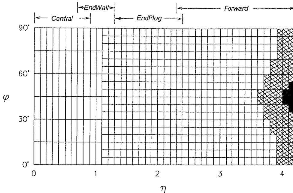
Figure 2.5: The CDF calorimeter segments shown in  $\eta - \phi$  plane. Hatched area shows partial depth coverage only due to cut for low beta quadrupoles. Black area shows no coverage.
