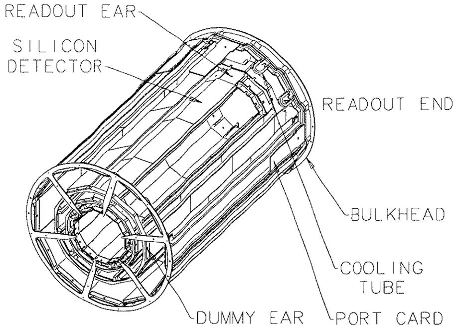
Figure 2.3: An isometric view of the SVX detector.  $r = 7.9 \text{ cm}$ ,  $l = \pm 25.5 \text{ cm}$ .
