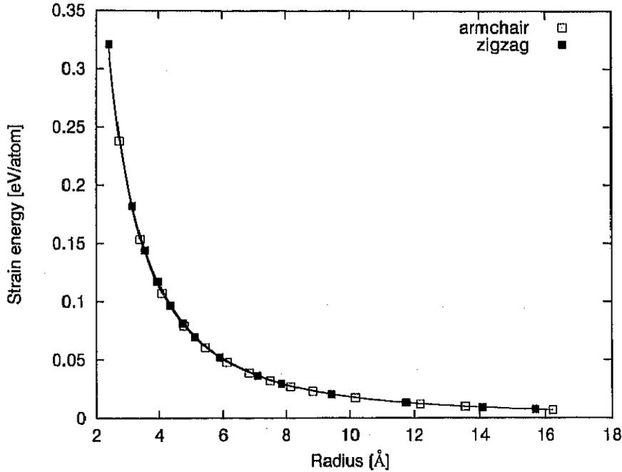
Figure 2.1: Strain energies per atom of the geometrically optimized armchair and zigzag NTs. The energy reference (zero energy) is the energy of a single graphite sheet. Open and solid squares indicate the  $E_{\text{strain}}^{(m,n)}$  of the armchair NTs and the zigzag NTs, respectively. The solid lines are least-square fitted curves with the form of  $A \times (\text{radius})^{-2}$ .
