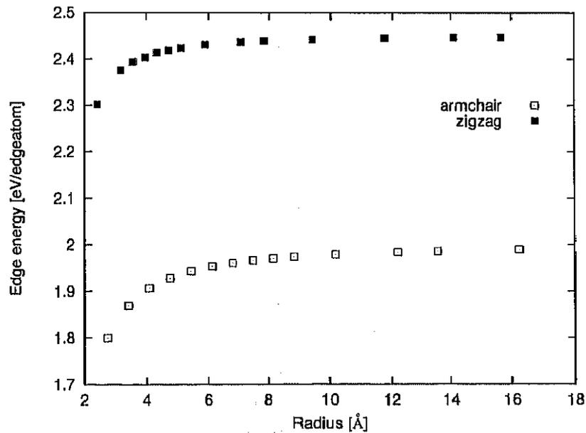
Figure 2.3: Edge formation energy per edge atom of the geometrically optimized armchair and zigzag NTs with finite lengths. Open and solid squares indicate the  $E_{\text{edge}}^{(m,n)}$  of the armchair and zigzag NTs, respectively.
