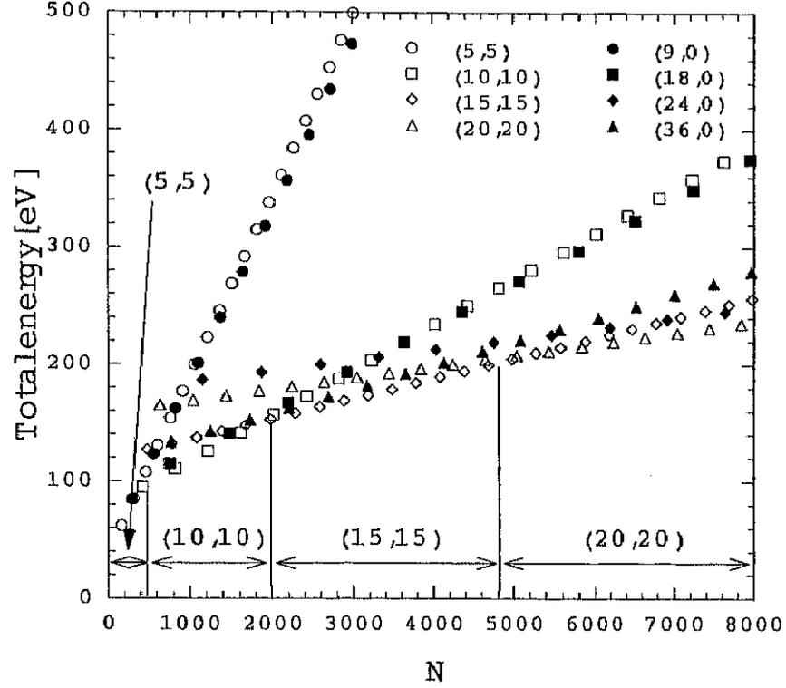
Figure 2.6: The total energy of a NT with finite length with respect to a flat graphite sheet as a function of  $N$ . We pick up eight kinds of NT from the armchair type,  $(5,5) \sim (20,20)$ , and from the zigzag type,  $(9,0) \sim (36,0)$ . The most stable tube is always of armchair type and its radius increases with increasing  $N$ . The most stable tube and its range of  $N$  are also indicated.
