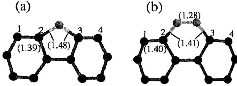
Figure 2.8: Side views of geometrically optimized pentagon and hexagon network on the armchair edge. Only top four rows and adatoms are depicted. Adatoms are indicated by lighter spheres. Numbers of 1 ~ 4 are atom indexes. Values in parentheses indicate the bond lengths in Å.
