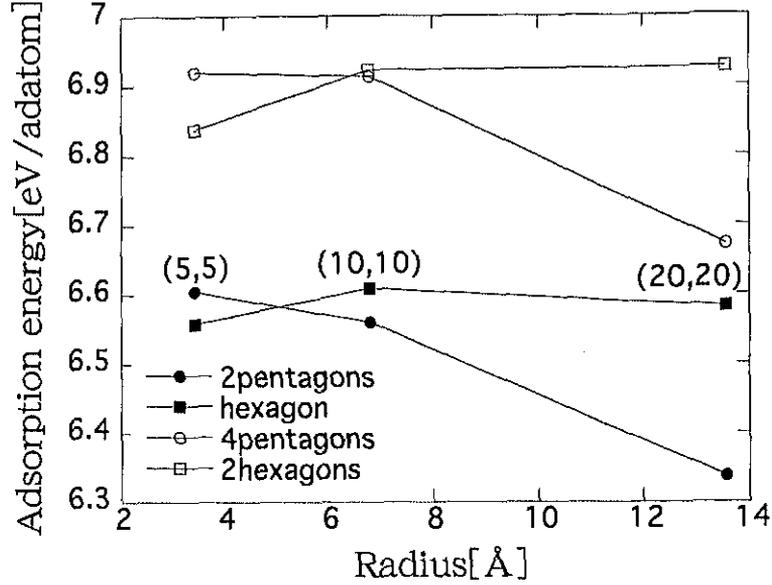
Figure 2.11: Adsorption energies of two pentagons, a hexagon, four pentagons and two hexagons on (5,5), (10,10) and (20,20) edge as a function of radius. The solid line is only a guide for eyes. For both cases of two and four pentagons, the adsorption energy decreases with increasing radius. The pentagon has high energy on the edge of the large radius NTs.
