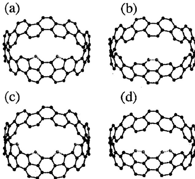
Figure 2.10: Structures of the geometrically optimized (10,10) edge with two or four adatoms. Only top 4 rows and adatoms are depicted. Adatoms are represented by lighter spheres. (a) Two adatoms form two-pentagon array. (b) Two adatoms form a hexagon. (c) Four adatoms form four-pentagon array. (d) Four adatoms form two-hexagon array. We construct similar structures on edges of the (5,5), (10,10) and (20,20) tubes to calculate the adsorption energies for each case.
