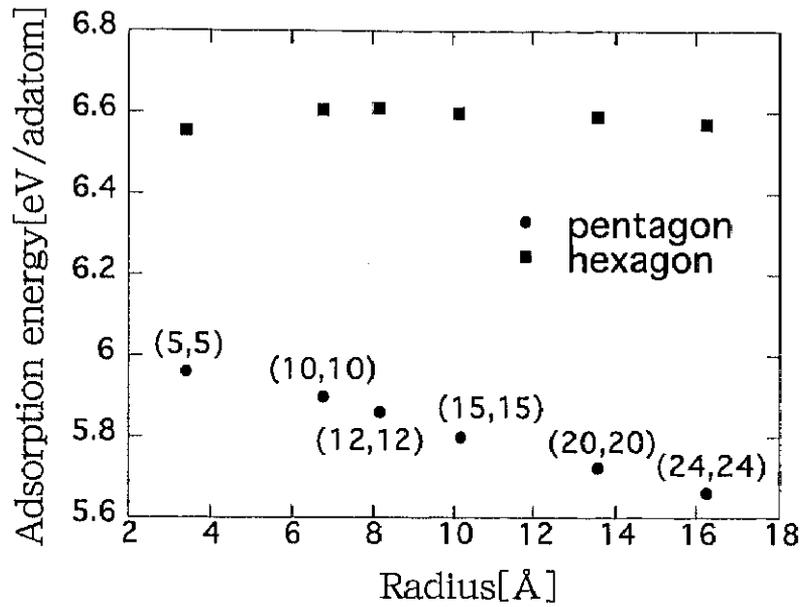
Figure 2.9: Adsorption energies on the armchair (5,5), (10,10), (12,12), (15,15), (20,20) and (24,24) edges. Solid circles and squares indicate the energies of the pentagon and hexagon network on the armchair edge, respectively.
