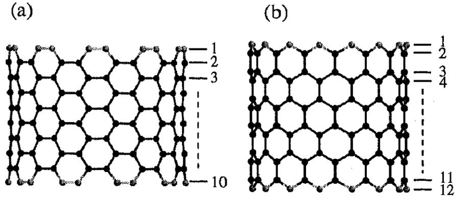
Figure 2.2: Side views of NTs with finite length used for calculations of edge formation energies. (a) An armchair NT is constructed from 10 rows. The  $(n, n)$ -tube here has  $20n$  atoms in total and  $4n$  atoms on the edge. (b) A zigzag NT is constructed from 12 rows. The  $(n, 0)$ -tube here has  $12n$  atoms in total and  $2n$  atoms on the edge. Atoms on the edge are depicted by lighter spheres.
