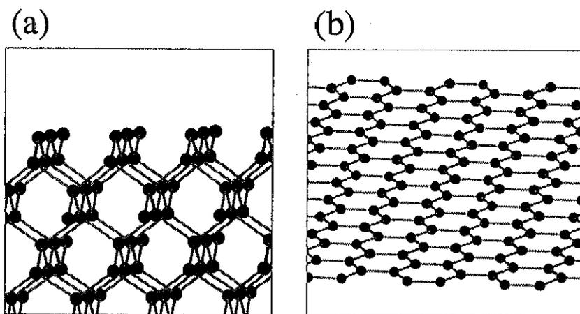
Figure 1.1: The networks of the carbon crystals are depicted. (a) Diamond: This 3-dimensional network is constructed only by the  $sp^3$  carbons. (a) Graphite: This 2-dimensional network is constructed only by the  $sp^2$  carbons.
