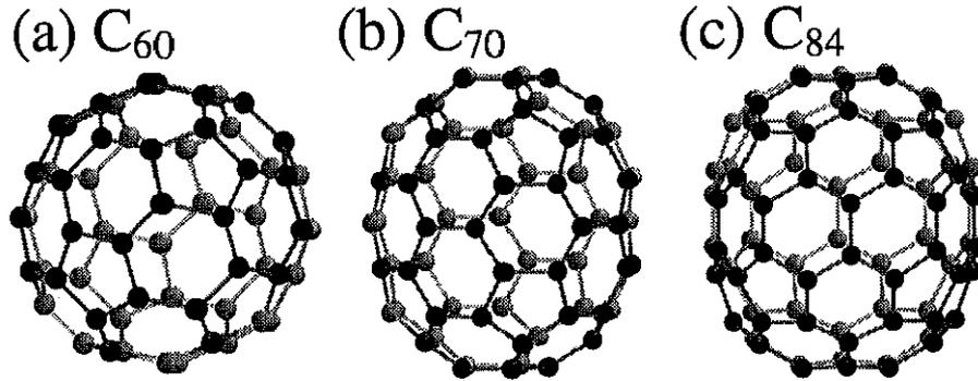
Figure 1.2: Three dimensional views of the close cage structures of the fullerenes. Atoms on the far side in these figures are indicated by the lighter spheres for clarity. We depict the  $C_{60}$  (a),  $C_{70}$  (b) and  $C_{84}$  (c), for example clusters of the fullerene family. These clusters are synthesized with relatively high yields.
