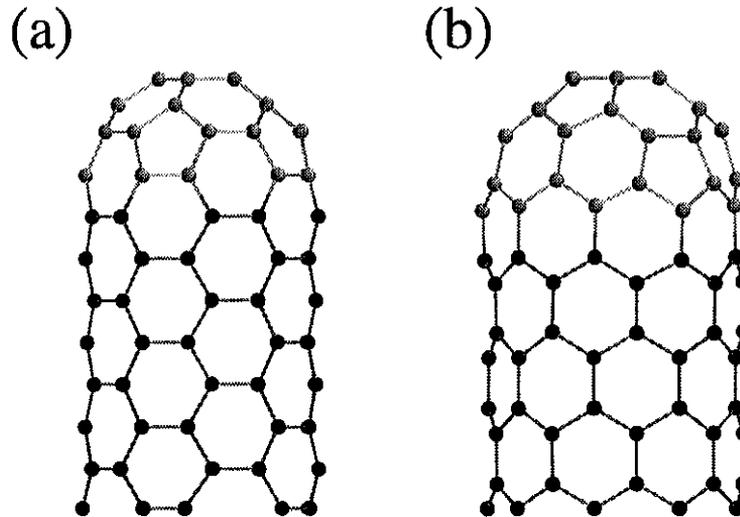
Figure 1.5: Side views of the two typical single-wall nanotubes with hemispheres of the fullerene  $C_{60}$  are depicted. For clarity, the atoms of the cap structures are indicated by the lighter spheres. (a) The armchair type nanotube: This nanotube is the (5,5)-tube. The cap structure is the  $C_{60}$  hemisphere with the pentagon on the top. (b) The zigzag type nanotube: This nanotube is the (9,0)-tube. The cap structure is the  $C_{60}$  hemisphere with the hexagon on the top.
