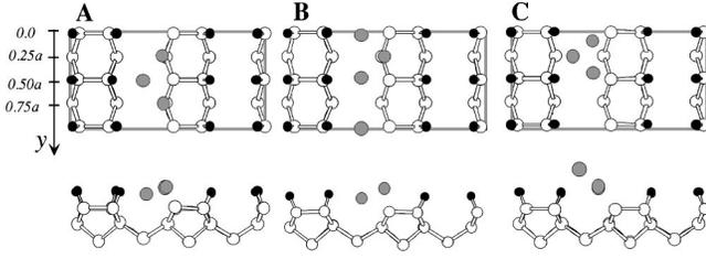
FIG. 1. Top and side views of optimized three atomic structures, A, B, and C, of a Ga wire on the hydrogenated Si(100) surface. White, shaded, and black circles denote Si, Ga, and H atoms, respectively.
