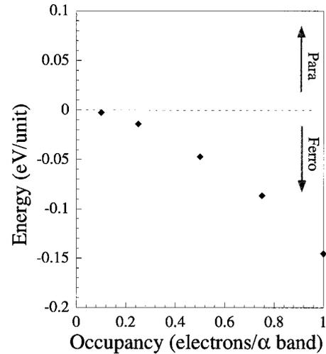
FIG. 4. Total-energy difference  $E_{\text{ferro}} - E_{\text{para}}$  between the paramagnetic and the ferromagnetic states as a function of the number of holes  $n_h$  doped in the flat band. The structure is fixed to the obtained structure C in Fig. 1.
