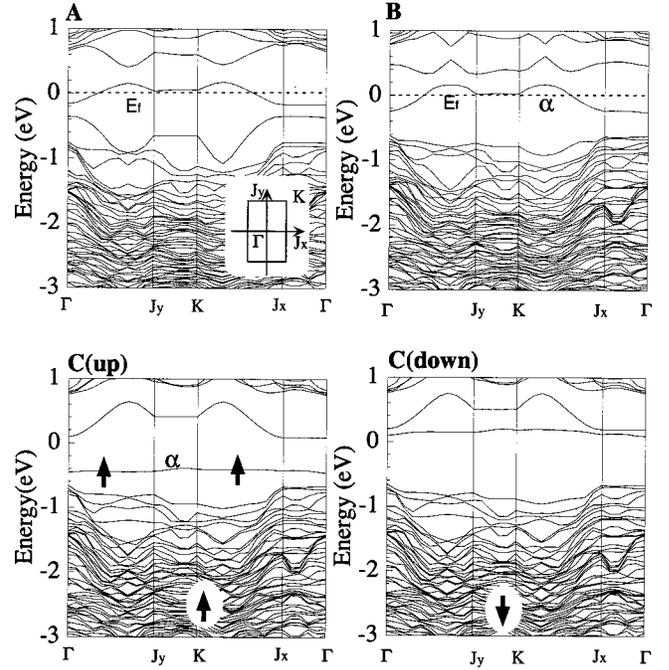
FIG. 2. Energy bands of a Ga wire on Si(100)/H with the atomic structures A, B, and C shown in Fig. 1. In the cases of A and B structures, the energy bands for up and down spins are degenerate. In the structure C, the highest occupied band splits by  $\sim 0.6$  eV for up and down spins, and the band only for the majority spin is occupied. The directions  $\Gamma - J_y$  and  $\Gamma - J_x$  are parallel and perpendicular, respectively, to the Ga wire.
