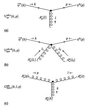
FIG. 1. Quark-gluon vertices needed for our one-loop calculations.
