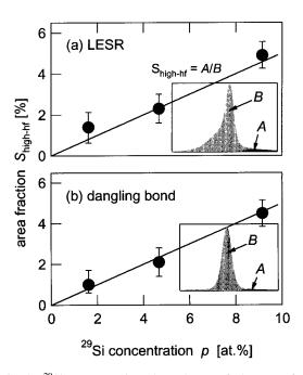
FIG. 4. <sup>29</sup>Si concentration dependence of the area fraction  $(S_{high-hf})$  of the high-field-side <sup>29</sup>Si hf line: (a) for LESR and (b) for dark ESR spectra.  $S_{high-hf}$  is given by the area ratio A/B.
