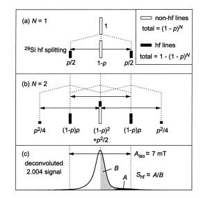
FIG. 6. Schematic views of <sup>29</sup>Si hf splitting for cases of (a) N = 1 and (b) N = 2, assuming two equivalent hf splittings. (c) Estimation of  $S_{\rm hf}$  and  $A_{\rm iso}$  for the deconvoluted 2.004 signal.
