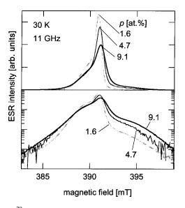
FIG. 3. <sup>29</sup>Si concentration dependence of the LESR spectrum of undoped a-Si:H. Intensities of those spectra are normalized to their areas. The upper and lower figures are linear and logarithmic plots, respectively.
