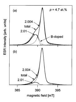
FIG. 5. Experimental deconvolution of two LESR signals for the case of p=4.7 at. %. Solid lines indicate the deconvoluted 2.004 and 2.01 spectra with high reliability in data analyses, while dashed lines include some ambiguity. Shaded regions show the high-field-side hf structure of <sup>29</sup>Si. The dark ESR spectrum of B-doped *a*-Si:H is also shown by a broken line.
