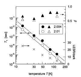
FIG. 2. Temperature dependence of  $T_1$  (circles) and  $\beta$  (triangles). The data were obtained for undoped *a*-Si:H with p = 4.7 at. %. Solid lines indicate the dependence  $T^{-3.4}$ . "LESR/dark" represents the ratio of peak heights of the LESR spectrum to the dark ESR spectrum.
