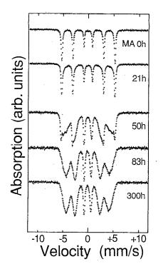
FIG. 5. <sup>57</sup>Fe Mössbauer spectra for the X=20 powders subjected to MA for different milling times.
