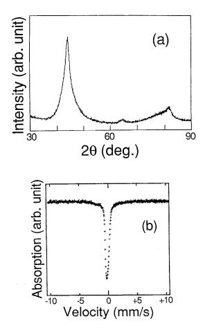
FIG. 8. (a) X-ray diffraction spectrum and (b)  $^{57}$ Fe Mössbauer spectrum for the X=50 powders ball milled in Ar gas for 200 h and further milled in N<sub>2</sub> gas atmosphere. Nitrogen content is 5.8 at. %.
