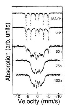
FIG. 3. <sup>57</sup>Fe Mössbauer spectra for the X=50 powders subjected to MA for different milling times.
