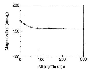
FIG. 4. Saturation magnetization as a function of milling time for the X=20 powders.
