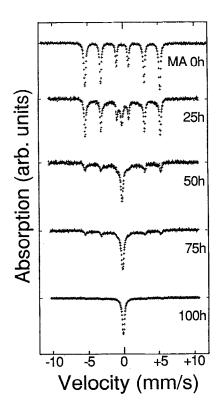
FIG. 6. <sup>57</sup>Fe Mössbauer spectra for the X = 70 powders subjected to MA for different milling times.
