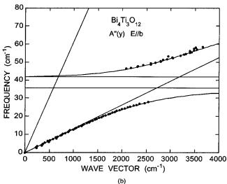
FIG. 5. Dispersion relations of phonon-polariton for a c-plate bismuth titanate crystal for the polarization along (a) the a axis and (b) the b axis. Closed circles denote observed values, and solid lines are calculated curves using Eq. (2).
