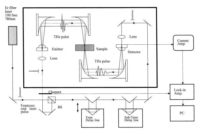
FIG. 1. Experimental setup of the THz time domain spectrometer.
