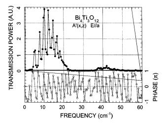
FIG. 3. The frequency-domain power and phase for the polarization  $E \parallel a$ .
