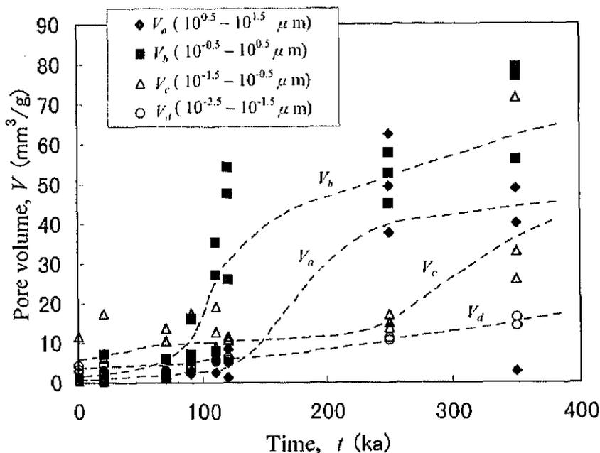
Fig. 15 Temporal changes in pore volume for four sub-ranges of pore size.
