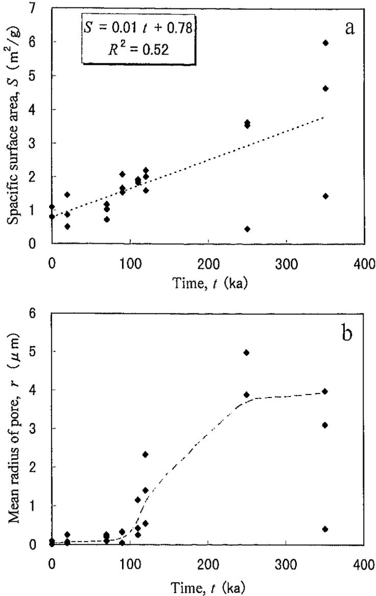
Fig. 16 Temporal changes in specific surface area,  $S$  (a), and mean pore radius,  $r$  (b).
