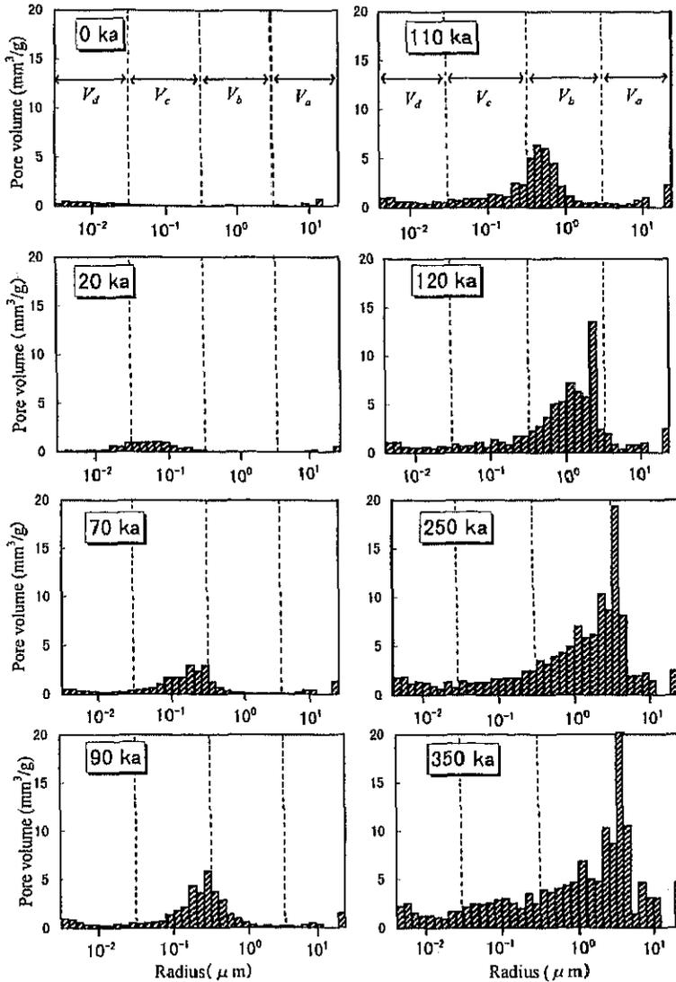
Fig. 14 Histograms of pore size distribution measured by the mercury intrusion porosimeter.
