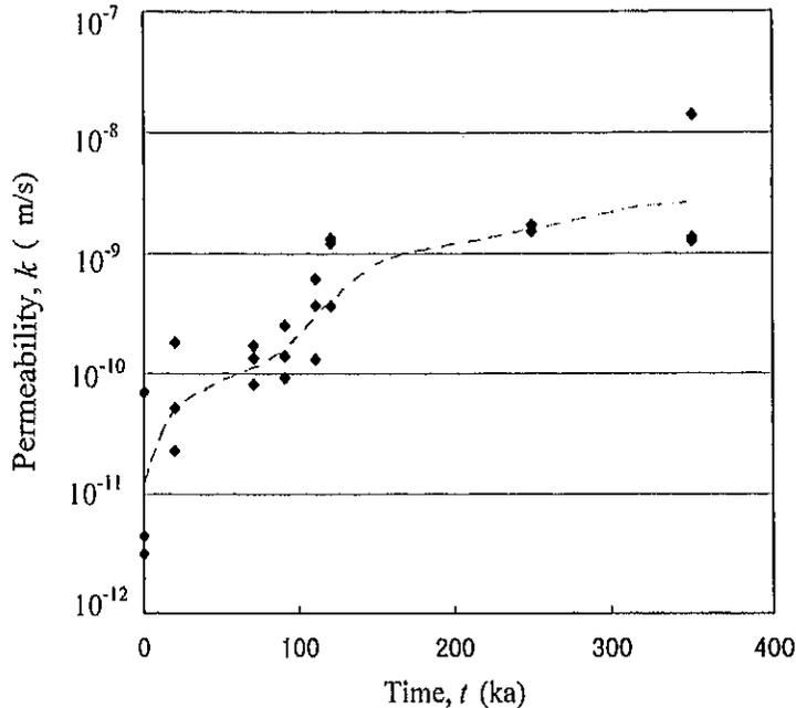
Fig. 17 Temporal changes in permeability using PSD data.
