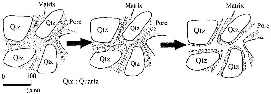
Fig. 25 Changes in pore structure of sandstone gravel.
