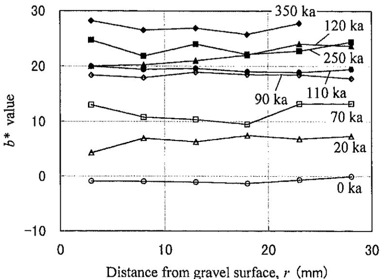
Fig. 10 Distribution of  $b^*$ -value measured on cutting surface of gravel.
