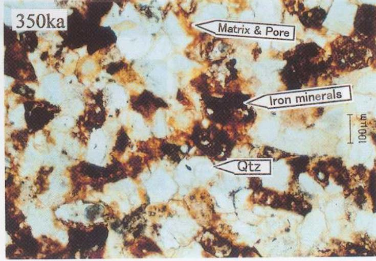
Fig. 7 Photomicrographs of sandstone in thin section (open nicols).
