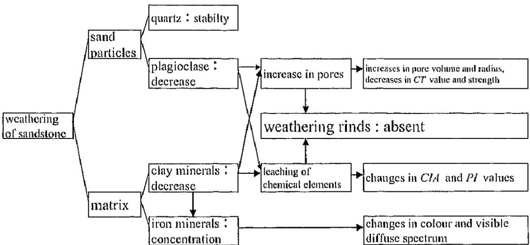
Fig. 27 General diagram of weathering mechanism of sandstone.
