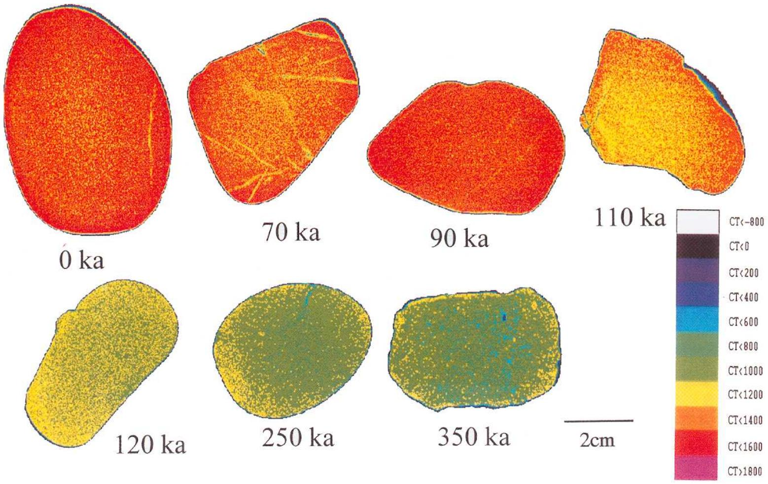
Fig. 18 Typical examples of X-ray CT images of sandstone gravel.
