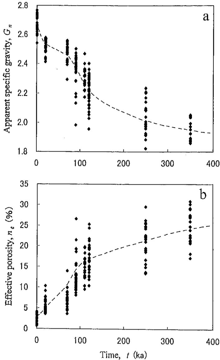
Fig. 13 Temporal changes in specific gravity,  $G_n$  (a), and effective porosity,  $n_e$  (b).
