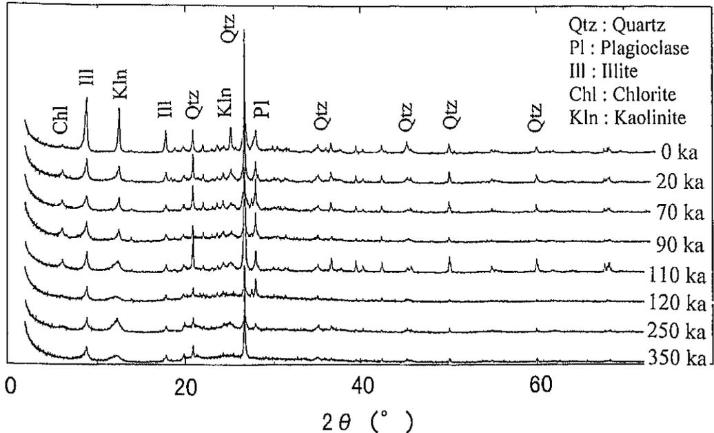
Fig. 8 X-ray diffraction patterns of matrix minerals in sandstone.
