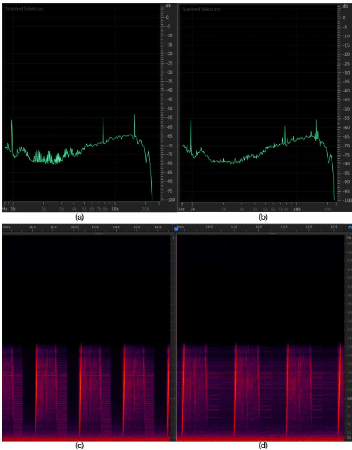
Figure 5.21: Comparison of the signal after noise removal and the signal without noise removal. Frequency spectrum (a) Signal with noise removed, (b) Signal without noise removed. Spectrogram (c) Signal from which noise has been removed, (d) Signal without noise removal.
