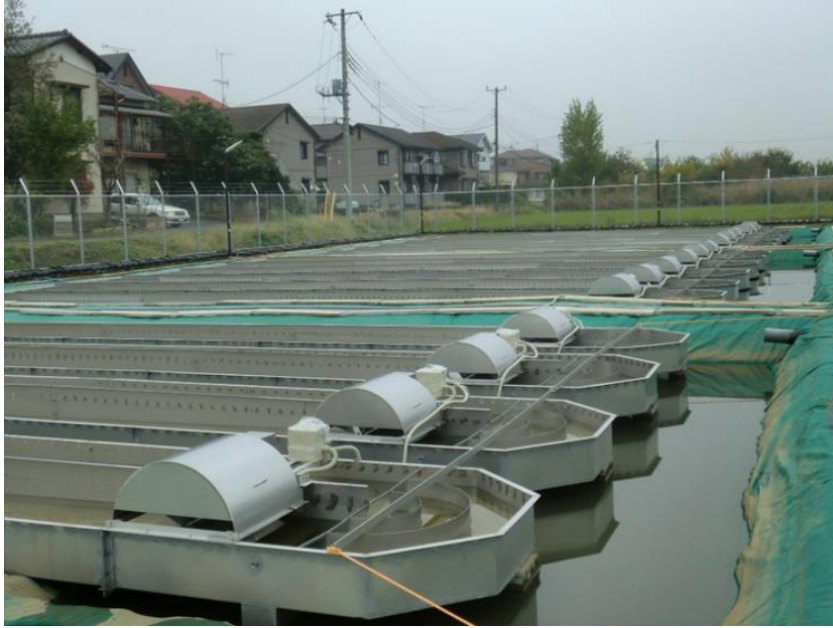
Figure 1-4 The photo of the open raceway pond [Source: Algae biomass and Energy System R&D Center (ABES)].
