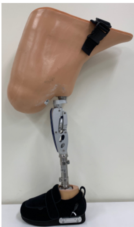
Figure 43 Multi-axial prostheses and simulated sockets used in the evaluation tests.
