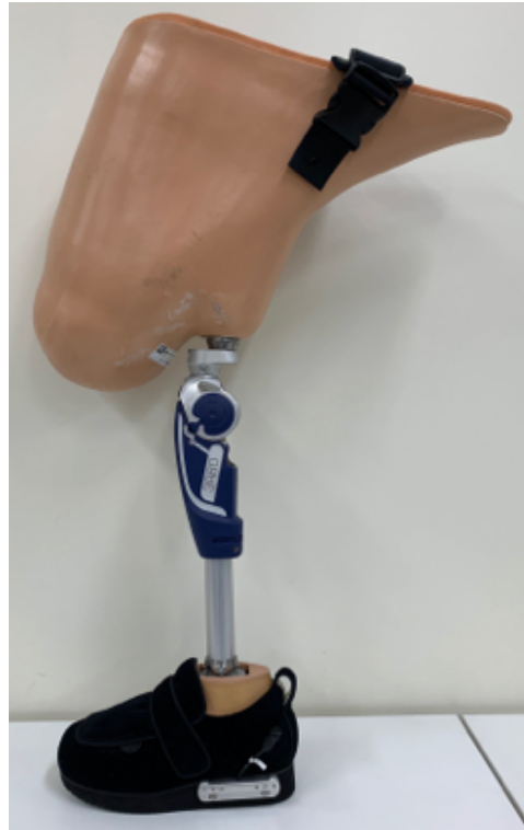
Figure 44 Single-axial prostheses and simulated sockets used in the evaluation tests.
