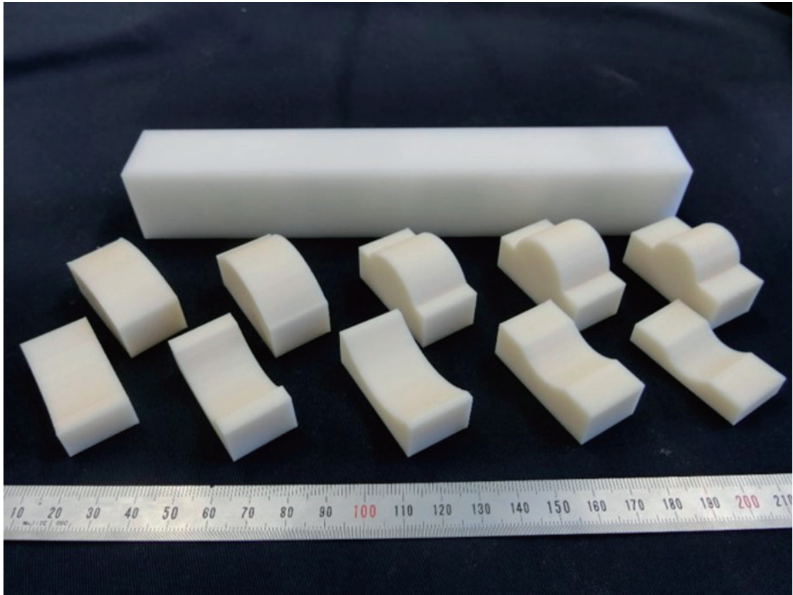
Fig. 2.4: Tactile sample with constant curvature
