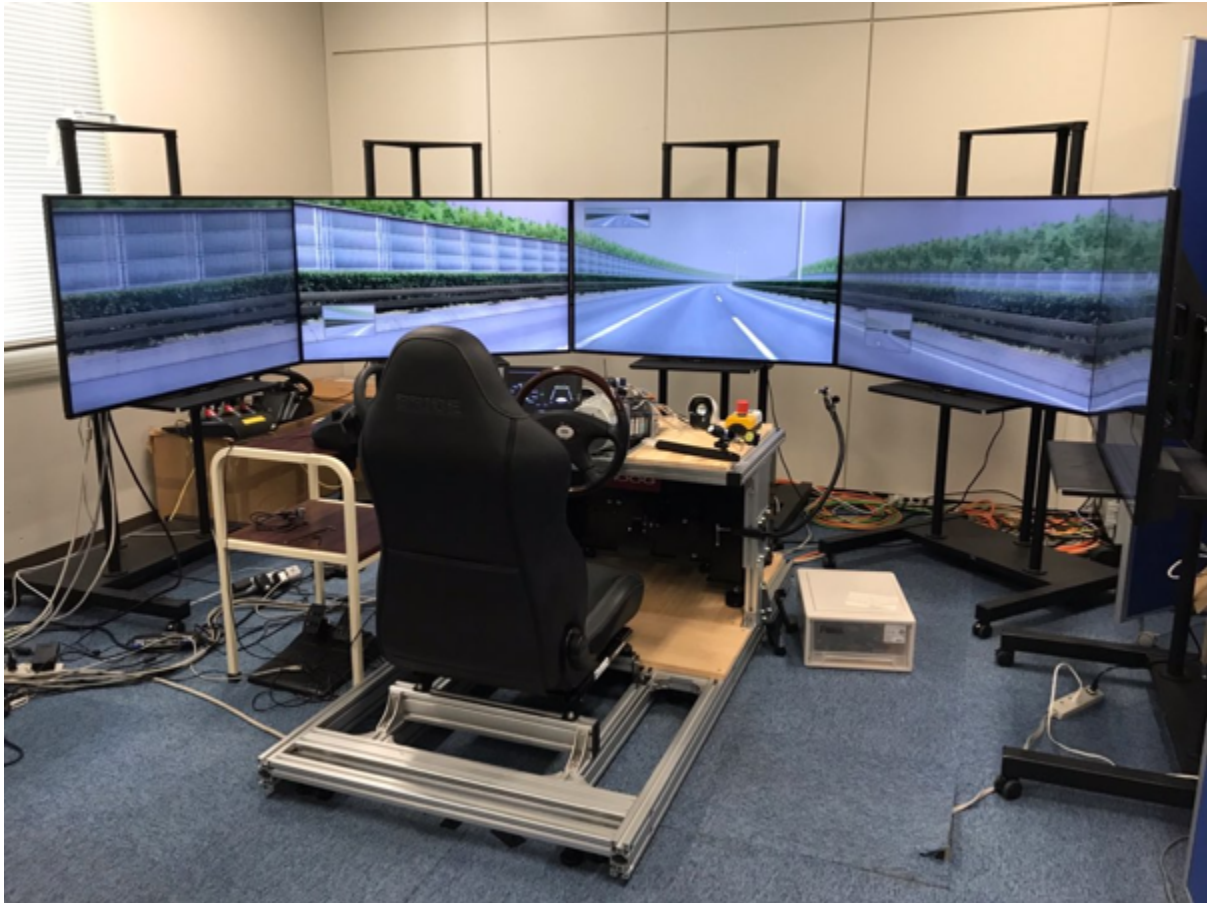
Figure 3.1 Fixed-base Driving simulator.
