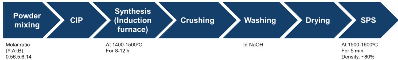
**Figure 3.2.** Flow chart of conventional synthesis process for bulk  $Y_xAl_yB_{14}$ . It consists of 7 steps, and the total process time is  $\geq 3$  days.
