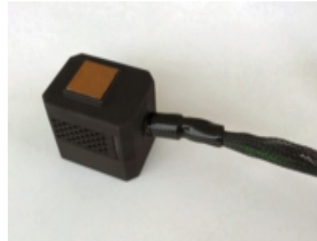
Figure 46. The thermo-electronic probe of the skin sensation threshold measurement device (Intercross-210, Intercross, Japan).
