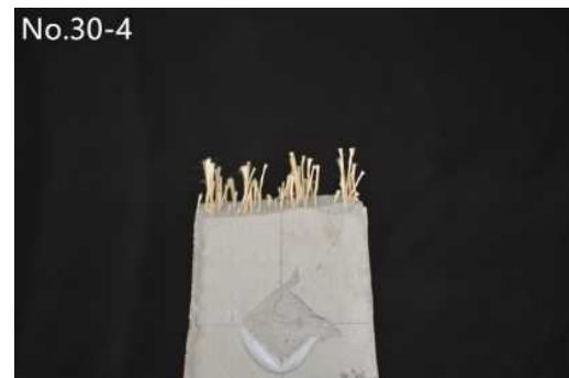
Fig. 2. 9 Final condition of cross section of aramid specimens
