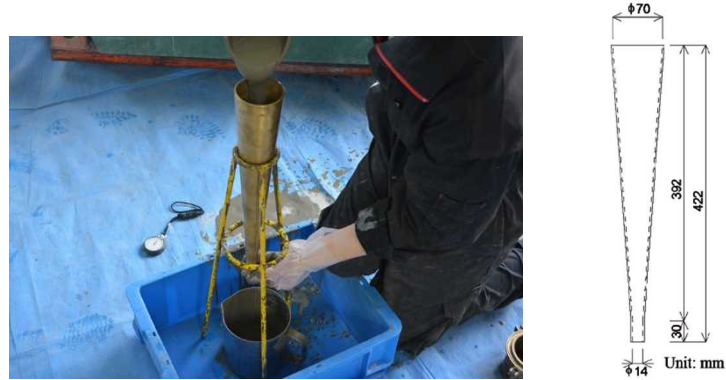
Fig. 2. 2 Flowability test using funnel
