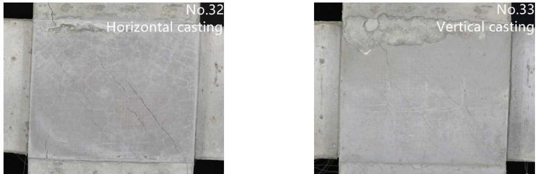
Fig. 4. 6 Crack pattern at maximum load (No.32 at 1/50rad., No.33 at 1/67rad.)
