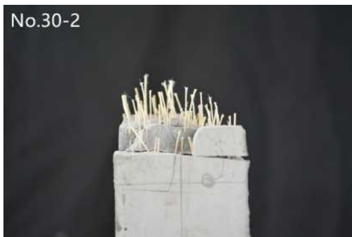
Fig. 2. 9 Final condition of cross section of aramid specimens
