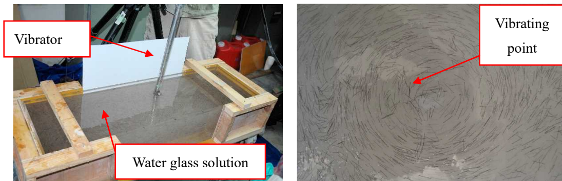
Fig. 4. 1 Example of fiber orientation after vibrating [4.4]
