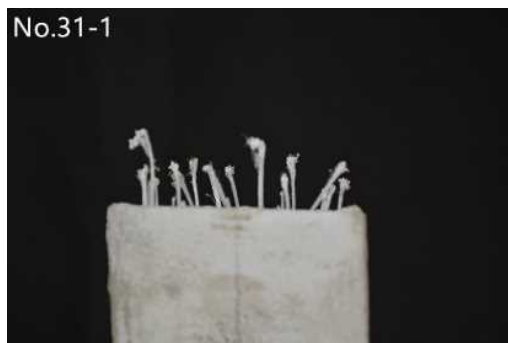
Fig. 2. 9 Final condition of cross section of aramid specimens
