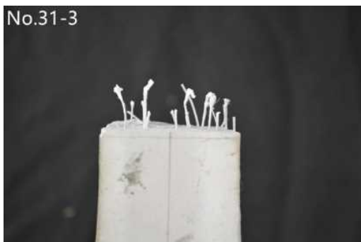
Fig. 2. 10 Final condition of cross section of PP specimens
