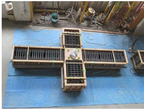
Fig. 3. 8 Install lateral reinforcements and the molds
