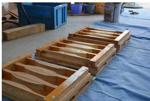
Fig. 2. 3 Molds for uniaxial tension test specimen
