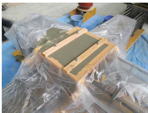
Fig. 3. 6 Casting the panel zone
