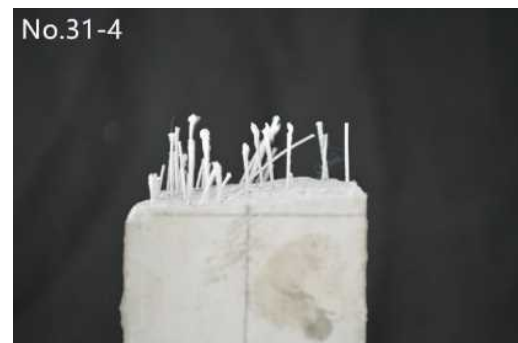
Fig. 2. 10 Final condition of cross section of PP specimens
