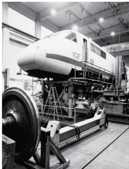
図 2.1: Vehicle test on a roller rig [62].
