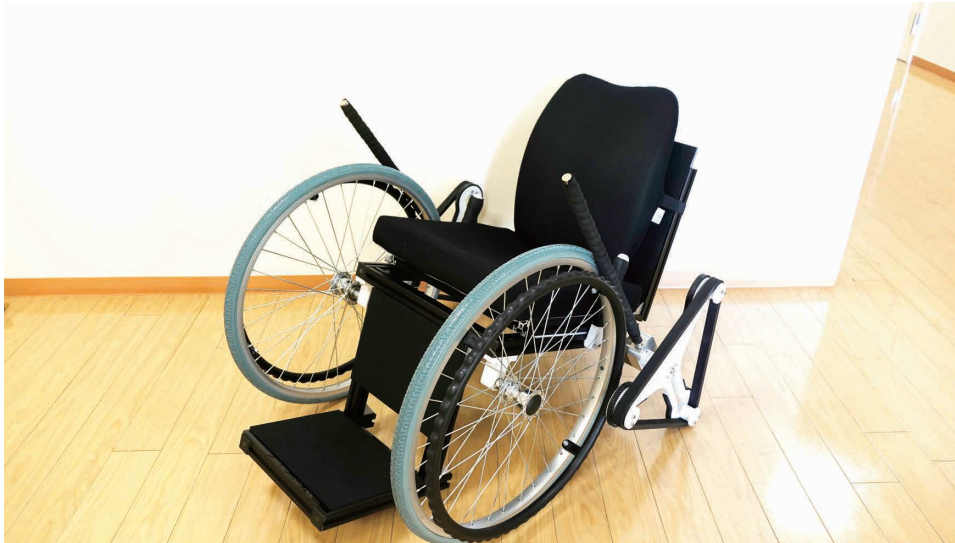
FIGURE 2.14: Overview of the developed second prototype of stair-climbing mobility device.
