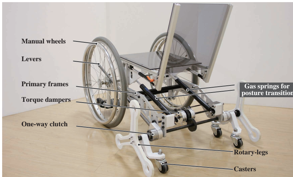
FIGURE 2.13: Overview of the developed first prototype of stair-climbing mobility device.
