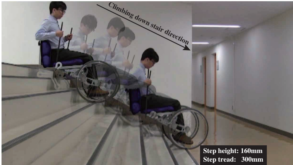
FIGURE 2.19: Experimental result of the climbing down the stair indoor.
