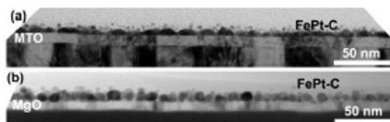
FIG. 9. Cross sectional TEM images of FePt granular films with 30 vol.% of C grown on (a) glass/a-NiTa (60 nm)/Cr (10 nm)/MTO (10 nm) and (b) glass/a-NiTa (60 nm)/MgO (10 nm) underlayers.
