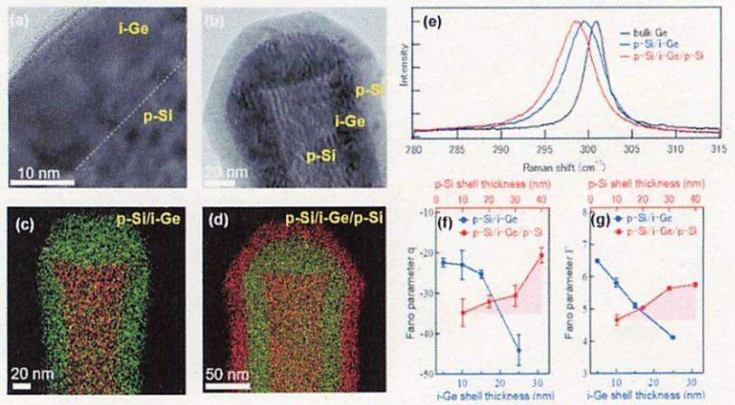
**Figure 7.** TEM and EDX mapping observed for (a) and (c) p-Si/i-Ge core-shell NWs, (b) and (d) p-Si/i-Ge/p-Si core-double shell NWs, (e) Ge optical phonon peaks observed for bulk-Ge, p-Si/i-Ge core-shell, and p-Si/i-Ge/p-Si core-double shell NWs, (f) q and (g)  $\Gamma$  observed for core-shell and core-double shell NWs.
