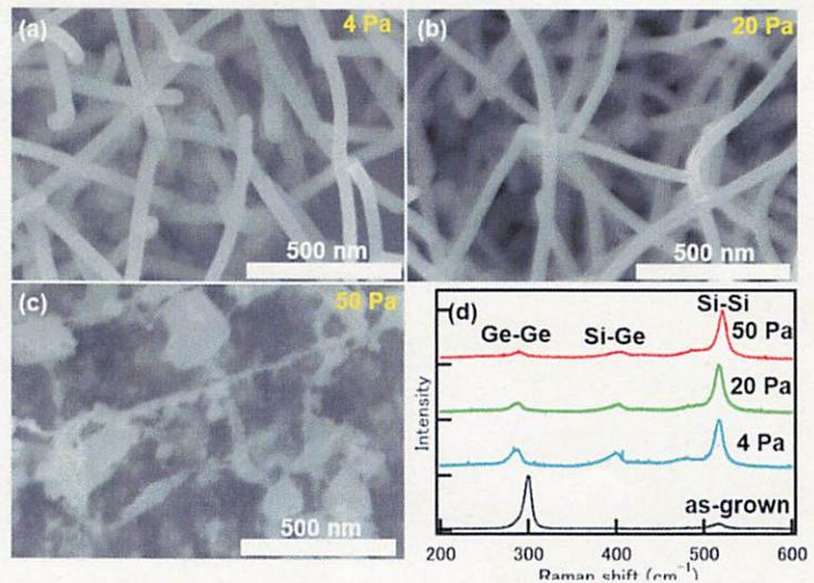
**Figure 9.** SEM images of i-Ge/p-Si NWs after RTA under  $\text{N}_2$  pressure of (a) 4 Pa, (b) 20 Pa, (c) 50 Pa at 800 °C. (d) Raman spectra of i-Ge/p-Si NWs.
