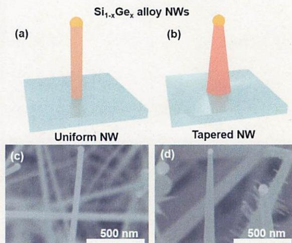
**Figure 11.** Schematic and SEM images of the  $\text{Si}_{1-x}\text{Ge}_x$  alloy NW (a), (c) uniform and (b), (d) tapered structure.
