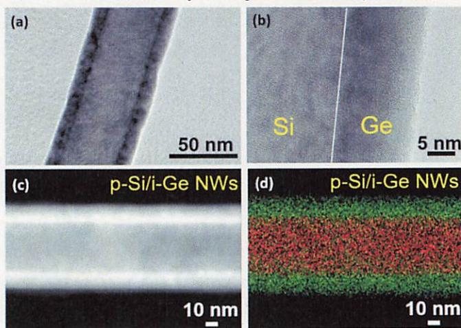
**Figure 2.** (a) Low and (b) high resolution TEM images of p-Si/i-Ge core-shell NW with a shell growth of 60 s. The scale bar of (a) and (b) are 50 nm and 5 nm, respectively. (c) STEM image and (d) EDX mapping with the scale bars of 10 nm. The red color and green colors are Si and Ge, respectively.
