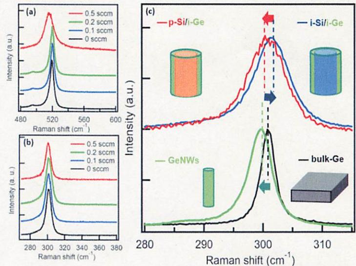
**Figure 3.** Raman spectra of p-Si/i-Ge core-shell NWs grown with B<sub>2</sub>H<sub>6</sub> fluxes from 0 sccm to 0.5 sccm observed for (a) Si optical phonon peaks and (b) Ge optical phonon peaks. (c) Ge optical phonon peaks compared to bulk-Ge, i-Ge NWs, i-Si/i-Ge core-shell NWs, and p-Si-i-Ge core-shell NWs.
