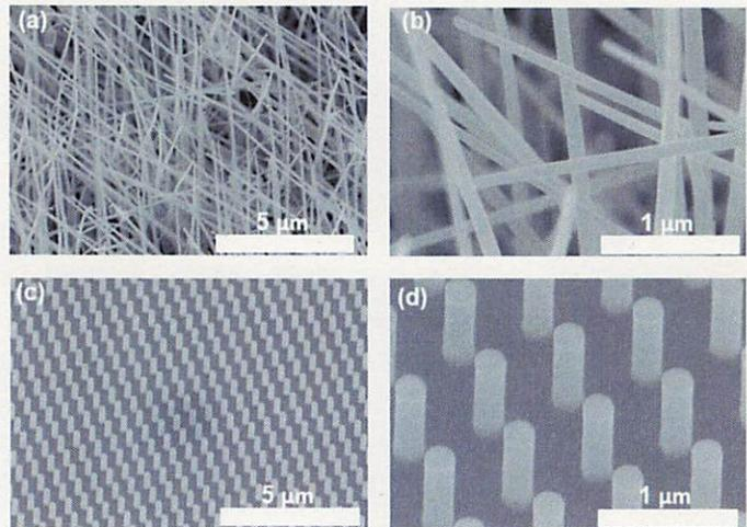
**Figure 4.** SEM images of Si NWs formed by (a), (b) bottom-up method, (c), (d) top-down method.
