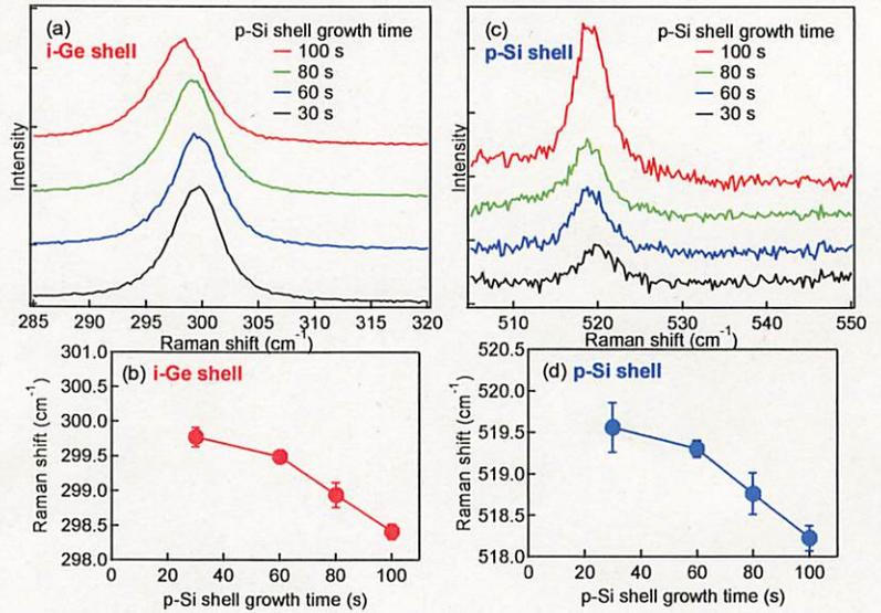
**Figure 6.** Raman spectra of p-Si/i-Ge/p-Si core-double shell NWs observed for various outer most p-Si shell growth times: (a) Ge and (c) Si optical phonon peaks and (b) Ge and (d) Si optical phonon peaks as a function of shell growth time.
