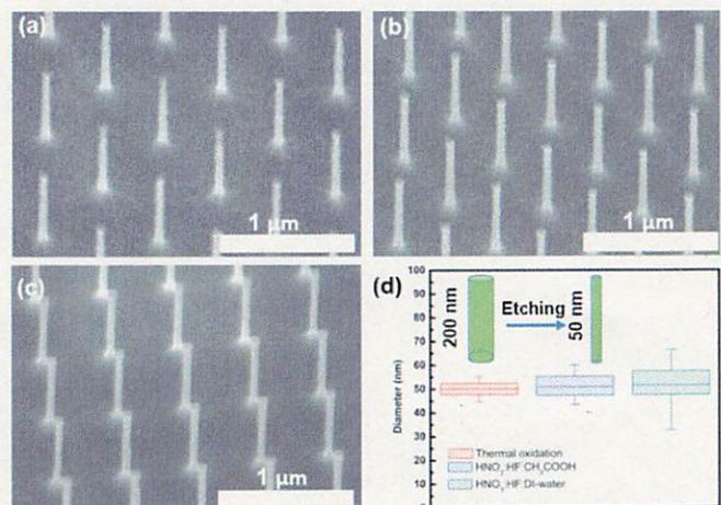
**Figure 5.** Si nanoarrays with the following conditions (a) HNO<sub>3</sub>/HF/DI (50:1:20) etching, (b) HNO<sub>3</sub>/HF/DI (400:1:20) etching, (c) thermal oxidation, (d) Si NW arrays diameter distribution.
