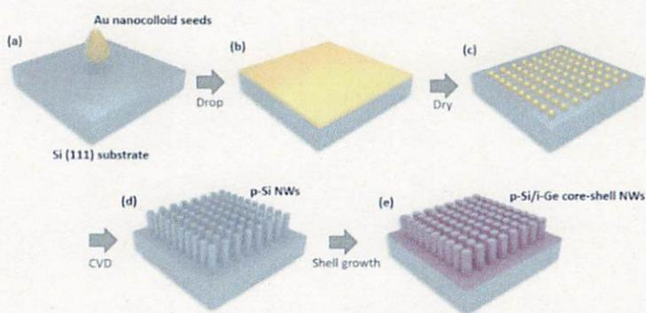
**Figure 1.** Schematic of the p-Si/i-Ge core-shell NW CVD growth process: (a)-(c) deposition of colloidal Au catalyst seeds on the Si (111) substrate; (d) formation of p-Si core NWs by SiH<sub>4</sub> gas flux; (e) final p-Si/i-Ge core-shell NWs.
