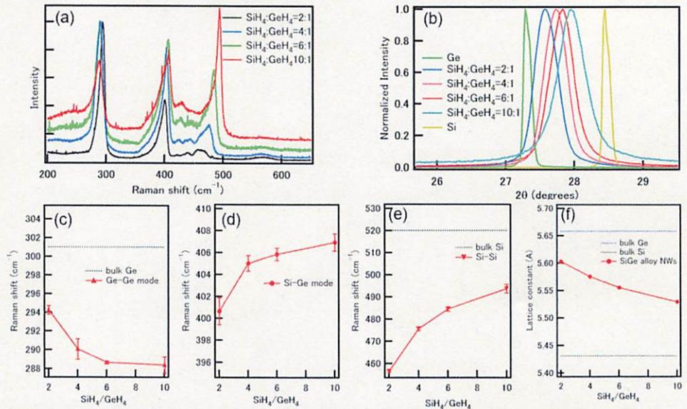
**Figure 13.** The varied ratios of  $\text{SiH}_4$  and  $\text{GeH}_4$  from 2:1 to 10:1 observed at (a) Raman spectra, (b) XRD; Raman peaks positions as a function of (c) Ge-Ge mode, (d) Si-Ge mode, (e) Si-Si mode; (f) lattice constants as a function of the varied ratios.
