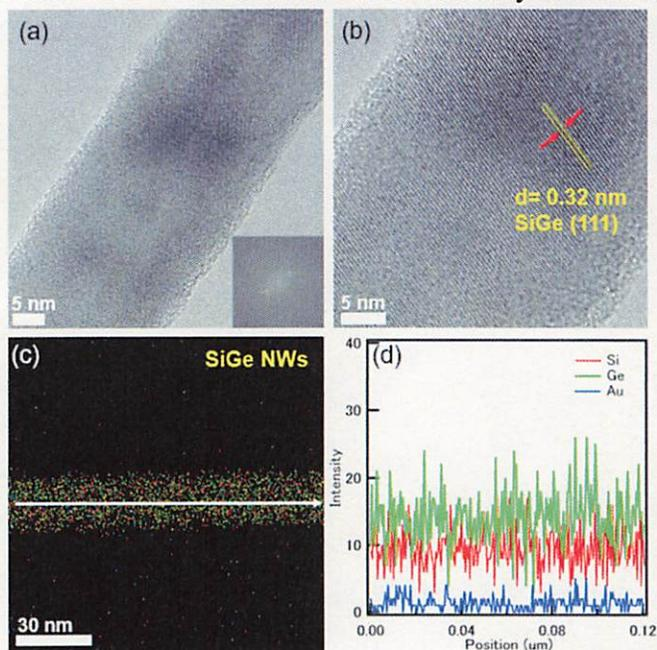
**Figure 12.** (a) and (b) high resolution TEM images of  $\text{Si}_{1-x}\text{Ge}_x$  alloy NWs. (Growth condition:  $\text{SiH}_4:\text{GeH}_4 = 10:1.7$ ; temperature:  $420^\circ\text{C}$ ). (c) EDX mapping, (d) line scan of the NWs.
