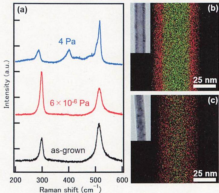
**Figure 10.** (a) Raman spectra of i-Ge/p-Si NWs observed for as-grown sample, the samples under the pressure of 4 Pa and  $6 \times 10^{-6}$  Pa annealing. TEM images and EDX mapping of (b) as-grown sample, (c) annealing sample.
