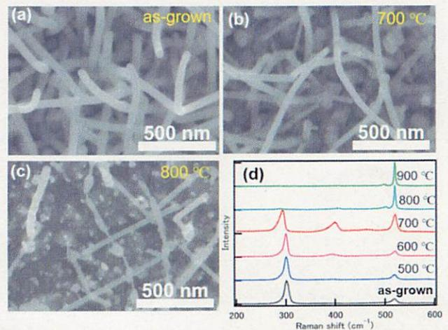
**Figure 8.** SEM images of i-Ge/p-Si NWs observed for (a) as-grown, samples after RTA AT (b) 700 °C, (c) 800 °C, (d) Raman spectra of i-Ge/p-Si NWs.
