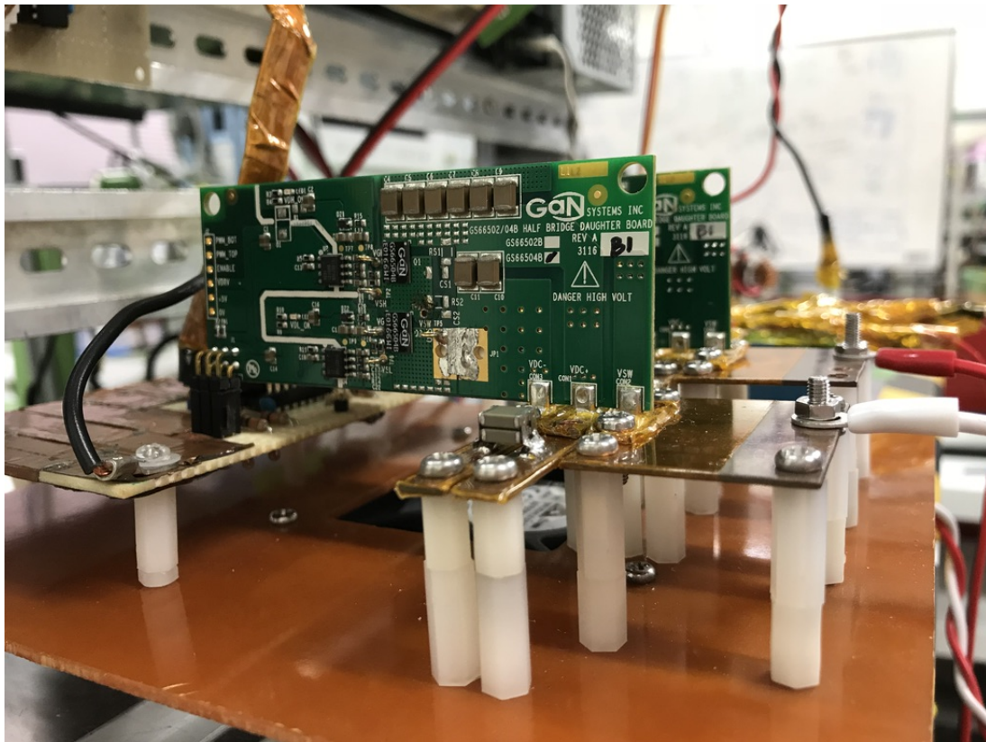
Fig. 4.29 Overview of H-bridge prototype with two evaluation boards from GaN Systems.
