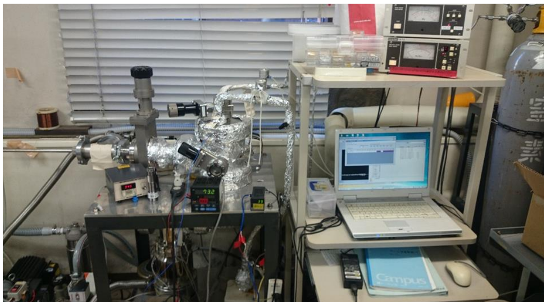
Figure 3.6.7: Schematic view of ALD system used in this study
