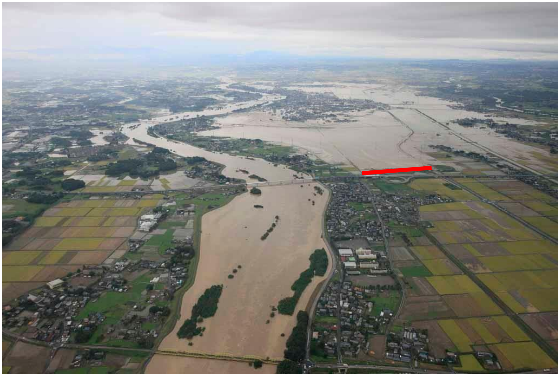
Figure 4-6 Photo shows road blocking floodwater by MTIL, 9 hours elapsed after the overflow, which is taken by the helicopter, an overview from the south-north angle.
