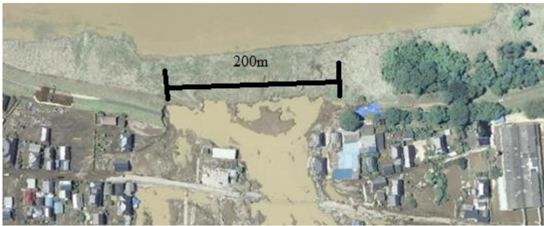
Figure 5-4 Levee breach (Image from GSI, edit by author)
