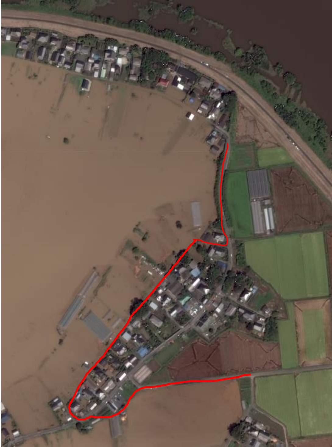
Figure 4-7 Photo shows road blocking floodwater by MTIL
