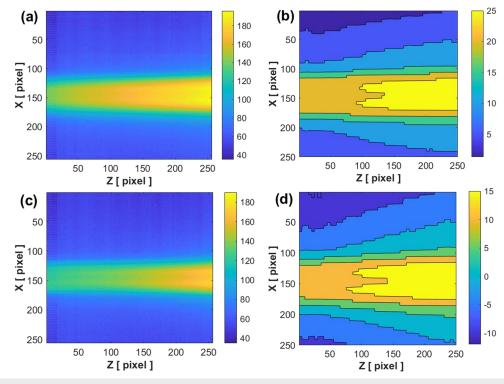
FIG. 7. (a), (c) and (b), (d) show the H $\alpha$  emission of 2D images and 2D image of PSD at B = 1.2 T and I = 100 A, and at B = 0.8 T and I = 120 A, respectively.
