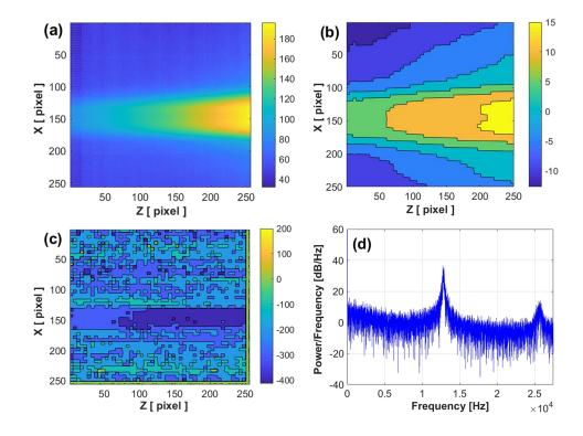
FIG. 5. (a), (b), (c) and (d) show the H $\alpha$  emission of 2D image, 2D image of PSD at the frequency of 13 kHz, 2D image of the phase angle of fluctuation at frequency of 13 kHz, and power spectrum of the fluctuation at pixel position of (X, Z) = (150, 250) on B = 0.8 T and I = 100 A, respectively.
