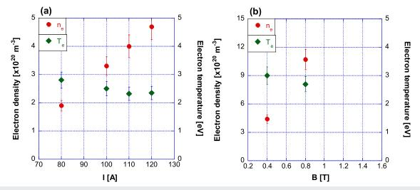
FIG. 9. (a) Shows the electron density and temperature against the discharge current at the magnetic field strength of 1.2 T and (b) shows them against the discharge current of 200 A measured by the Thomson scattering system settled at #1 port.
