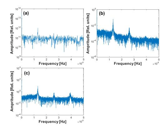
**FIG. 4**. (a), (b) and (c) show the FFT analysed spectra of the line integrated density,  $H\alpha$  emission detector, and the target plate potential, respectively.
