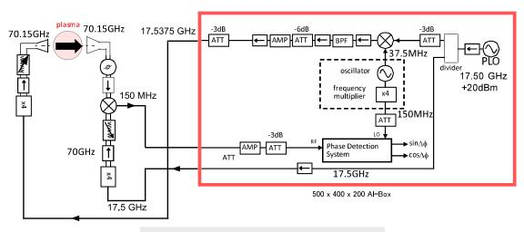
FIG. 2. The frequency multiplied microwave interferometer system.
