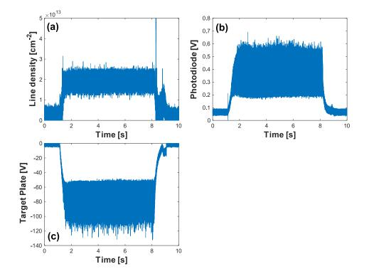
FIG. 3. (a) Line density, (b)  $H\alpha$  line emission and (c) target plate voltage on the plasma at the conditions of B = 0.8 T and I = 80 A.
