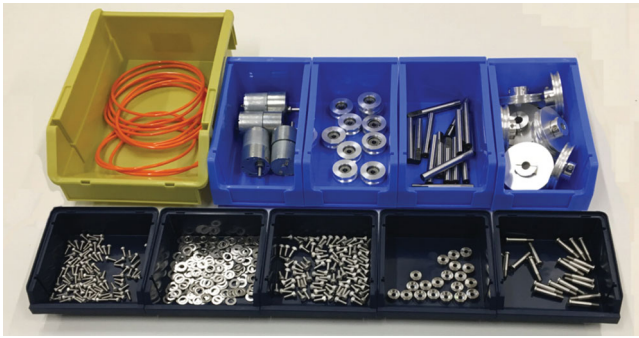
Figure 7. Example of 10 parts bins.
