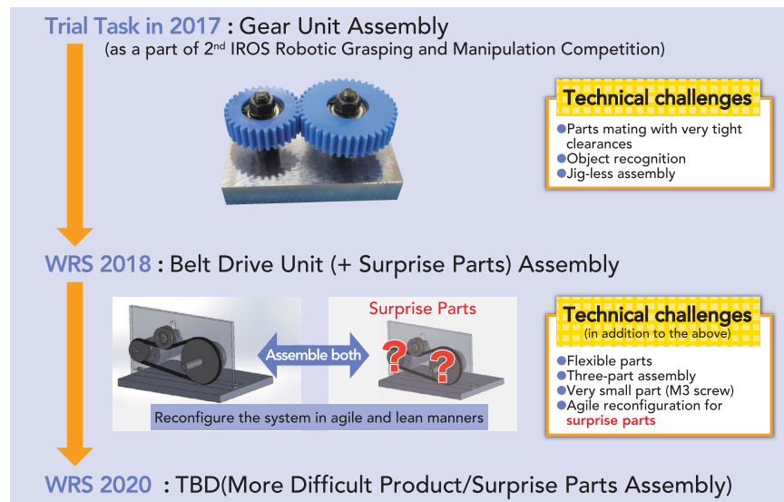
Figure 2. Milestones of the Assembly Challenge.
