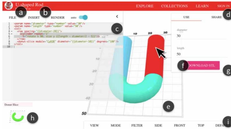
Figure 5.4: Cloud-based design platform[47]. CraftML offers a rich set of programming features familiar to web developers of all skill levels. This design platform also function as design repository. It is easily accessible to CraftML users and share both the model and its programming code.
