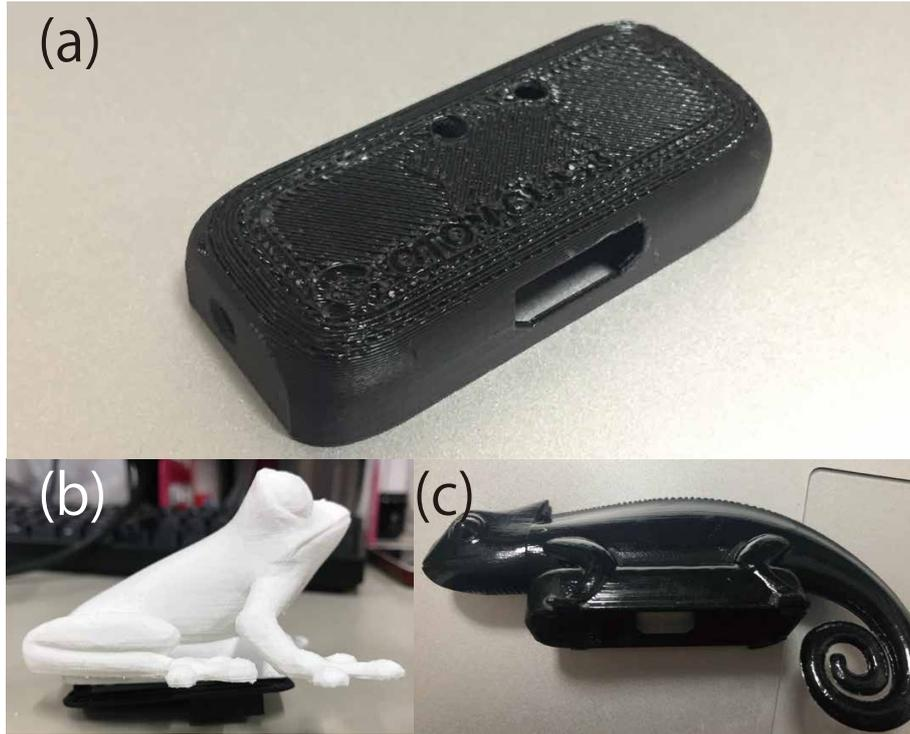
Figure 4.3: (a) The cabinet of OtonGlass printed by 3D-printer of Fused Deposition Modeling (FDM). (b) and (c) mean 3D-printed samples in Figure 4.4. (b) Frog was 3D-printed by Makerbot Replicator and (c) chameleon was 3D-printed by formlabs Form2 <sup>2</sup><https://formlabs.com>
