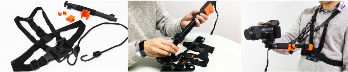
Figure 3.4: Left: all of parts we prepared. They consists of a monopod, harness, bungee code, and 3D-printed components. Center: assembly phase of these parts. Right: the user is equipped with our instrument.
