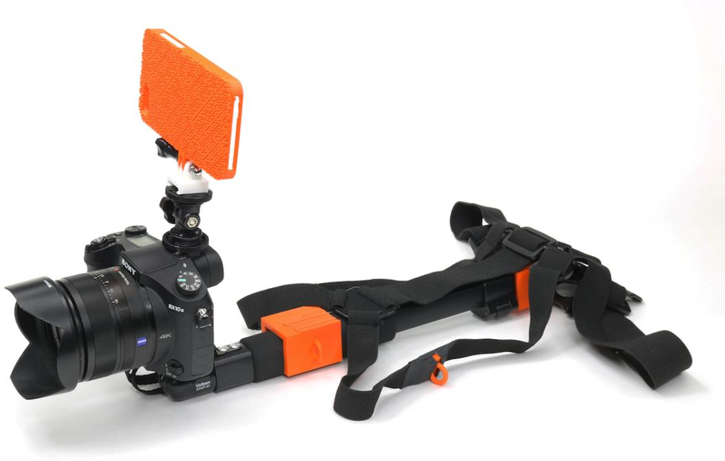
Figure 3.2: our instrument assembling some parts consisted of ready-made goods and components printed with a 3D printer
