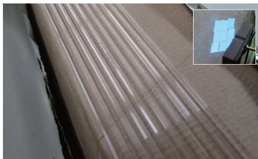
Fig. 1. Photograph of nine scintillating fibers forming a plane. The inset shows the cross section of the nine fibers before being connected to the MPPC.
