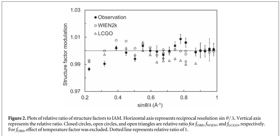
**Figure 2.** Plots of relative ratio of structure factors to IAM. Horizontal axis represents reciprocal resolution  $\sin \theta / \lambda$ . Vertical axis represents the relative ratio. Closed circles, open circles, and open triangles are relative ratio for  $f_{\text{OBS}}$ ,  $f_{\text{WIEN}}$ , and  $f_{\text{LCGO}}$ , respectively. For  $f_{\text{OBS}}$ , effect of temperature factor was excluded. Dotted line represents relative ratio of 1.
