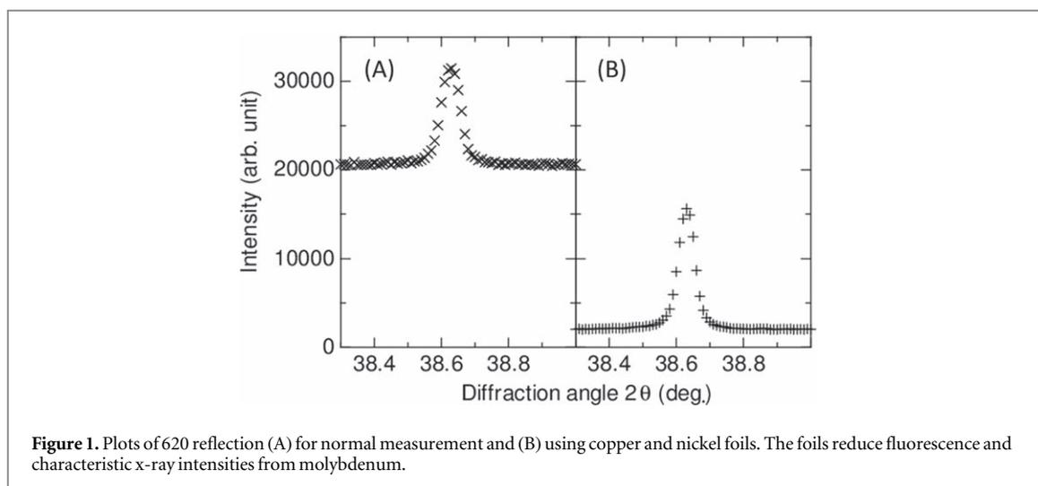
**Figure 1.** Plots of 620 reflection (A) for normal measurement and (B) using copper and nickel foils. The foils reduce fluorescence and characteristic x-ray intensities from molybdenum.
