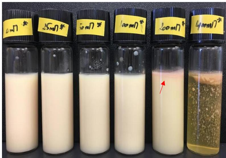
Figure 24. Effect of NaCl concentration (0-400 mM) on the visual appearance of 5% (w/w) soybean O/W emulsions prepared using purified glycyrrhizin (GA) or licorice root extract (LRE), at constant glycyrrhizin concentration (0.1%, w/w) and pH7
