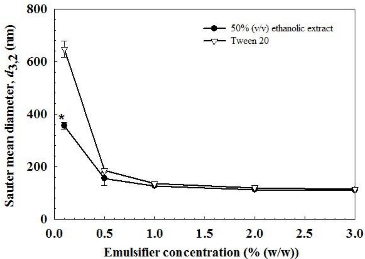
Figure 3. Effect of emulsifier concentration on the Sauter mean diameter ( $d_{3,2}$ ) of 10% (w/w) soybean O/W emulsions prepared using a high-pressure homogenizer (100 MPa, 4 passes). \*A small layer of oil was observed on the top of this sample.
