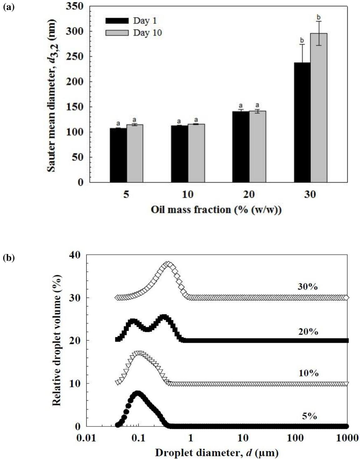
Figure 5. Effect of oil mass fraction on (a) the Sauter mean diameter ( $d_{3,2}$ ) and (b) droplet size distributions of soybean O/W emulsions containing 2% (w/w) of 50% (v/v) ethanolic extract.
