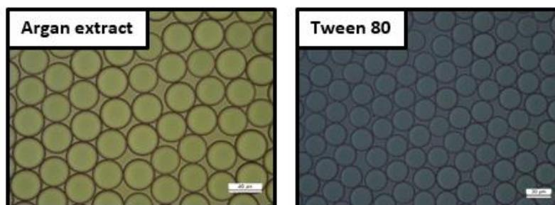
Figure 18. Droplet size distribution and optical micrographs of prepared emulsions in WMS 11-1 using 1% (w/w) argan extract or Tween 80.
