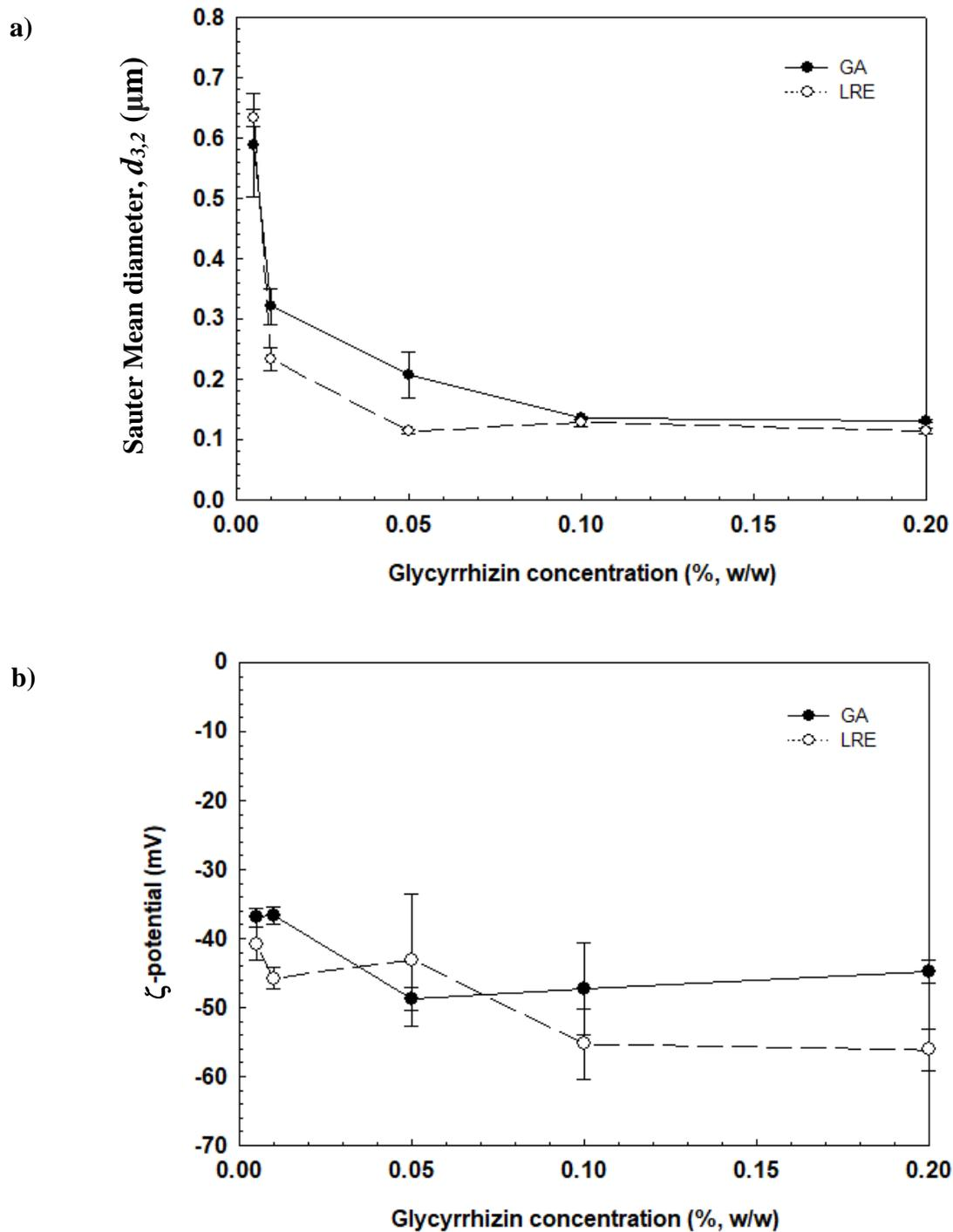
Figure 21. Effect of glycyrrhizin concentration in continuous phase on (a) volume mean diameter ( $d_{4,3}$ ) and (b) the  $\zeta$ -potential of emulsions prepared using purified glycyrrhizin (GA) or licorice root extract (LRE) at pH 7.
