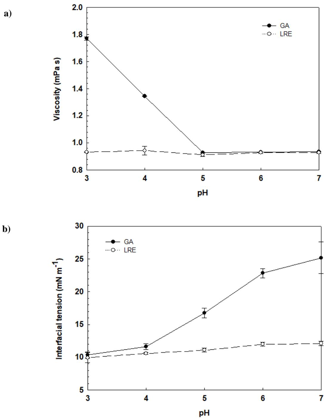
Figure 20. Effect of pH on the (a) viscosity and (b) interfacial tension of licorice root extract (LRE) and purified glycyrrhizin (GA), at constant glycyrrhizin concentration (0.1%, w/w). The interfacial tension between Milli-Q water and oil was  $26.2 \pm 0.7 \text{ mN m}^{-1}$ , at  $25 \text{ }^\circ\text{C}$ .
