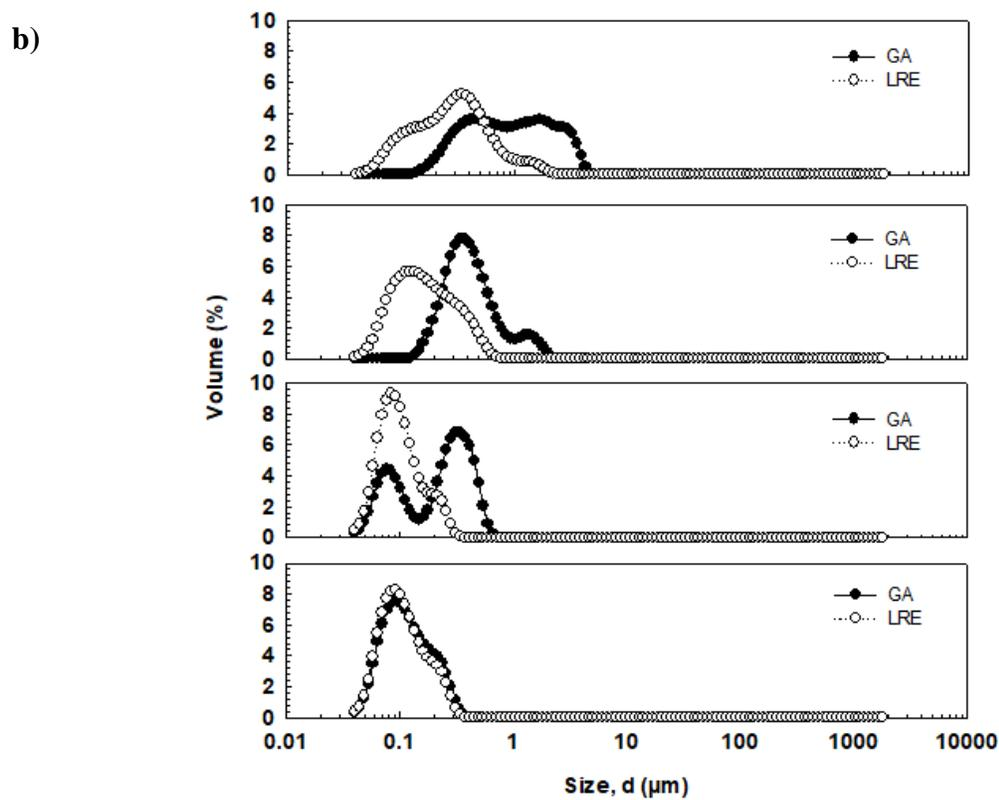
Figure 22. Effect of oil mass fraction on (a) the volume mean diameter ( $d_{4,3}$ ) and (b) the droplet size distribution of soybean O/W emulsions prepared using purified glycyrrhizin (GA) or licorice root extract (LRE), at constant glycyrrhizin concentration (0.1%, w/w) and pH 7.
