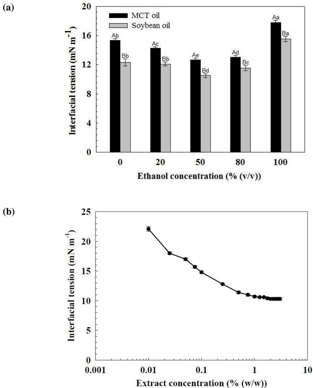
Figure 1. Effect of the extraction solvent on the interfacial tension of newly created interfaces. (a) Effect of extract type (1% (w/w)) on the interfacial tension at the oil/water interface. (b) Interfacial tension as a function of 50% (v/v) ethanolic extract concentration at the soybean oil/water interface. The interfacial tension between milli-Q water and oil was  $26.8 \pm 0.2$  and  $26.3 \pm 0.1$  for MCT oil and soybean oil respectively.
