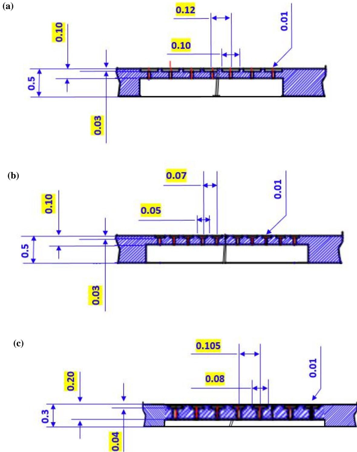
Figure 12. Cross-sectional representation of MC array chips used in this study: (a) WMS 1-2, (b) WMS 1-3 and (c) WMS 11-1. Variable dimensions (mm) are highlighted in yellow.
