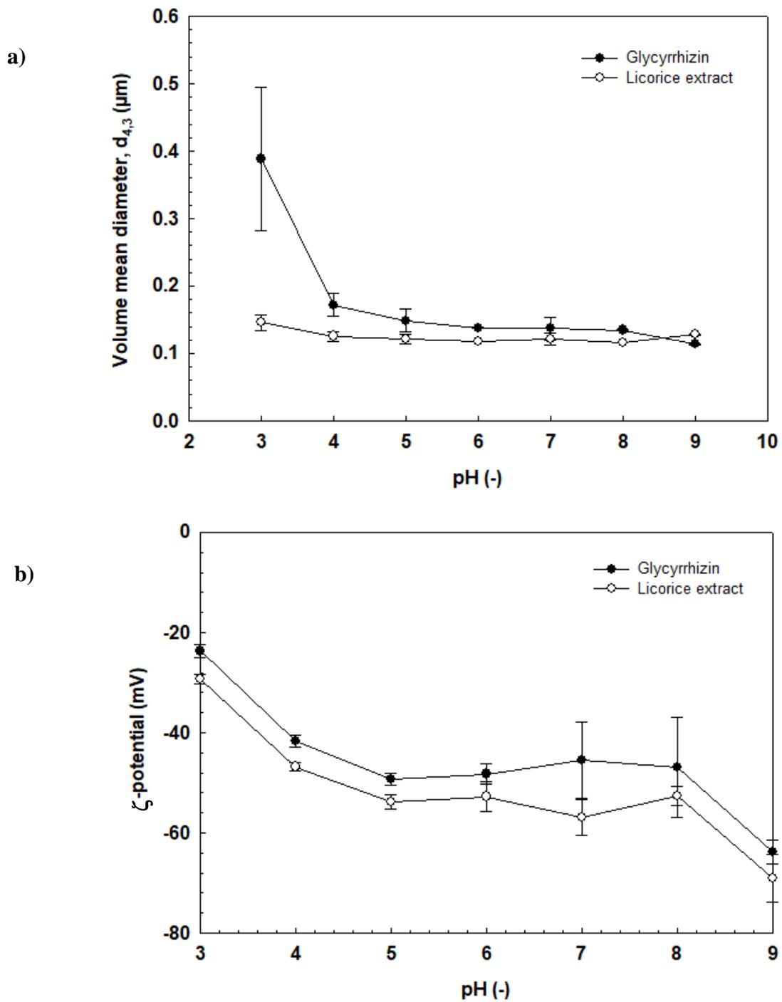
Figure 23. Effect of pH on (a) the volume mean diameter ( $d_{4,3}$ ) and (b) the  $\zeta$ -potential of 5% (w/w) soybean O/W emulsions prepared using purified glycyrrhizin (GA) or licorice root extract (LRE), at constant glycyrrhizin concentration (0.1%, w/w) and pH 7.
