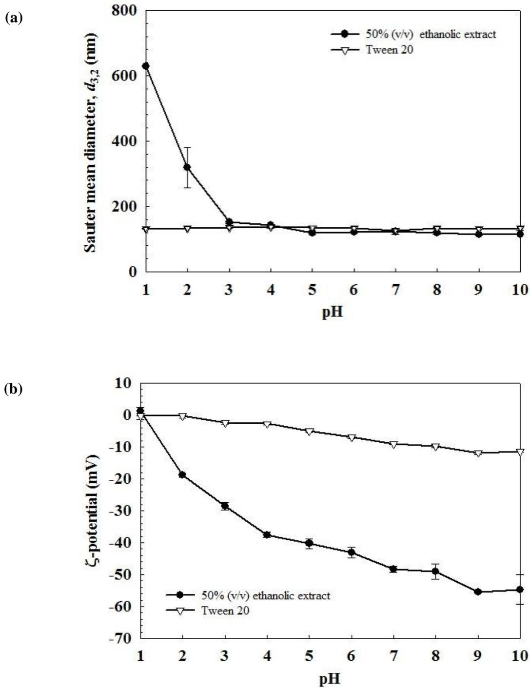
Figure 7. Effect of pH on (a) the Sauter mean diameter ( $d_{3,2}$ ) and (b)  $\zeta$ -potential of 10% (w/w) soybean O/W emulsions containing 2% (w/w) of Tween 20 or 50% (v/v) ethanolic extract.
