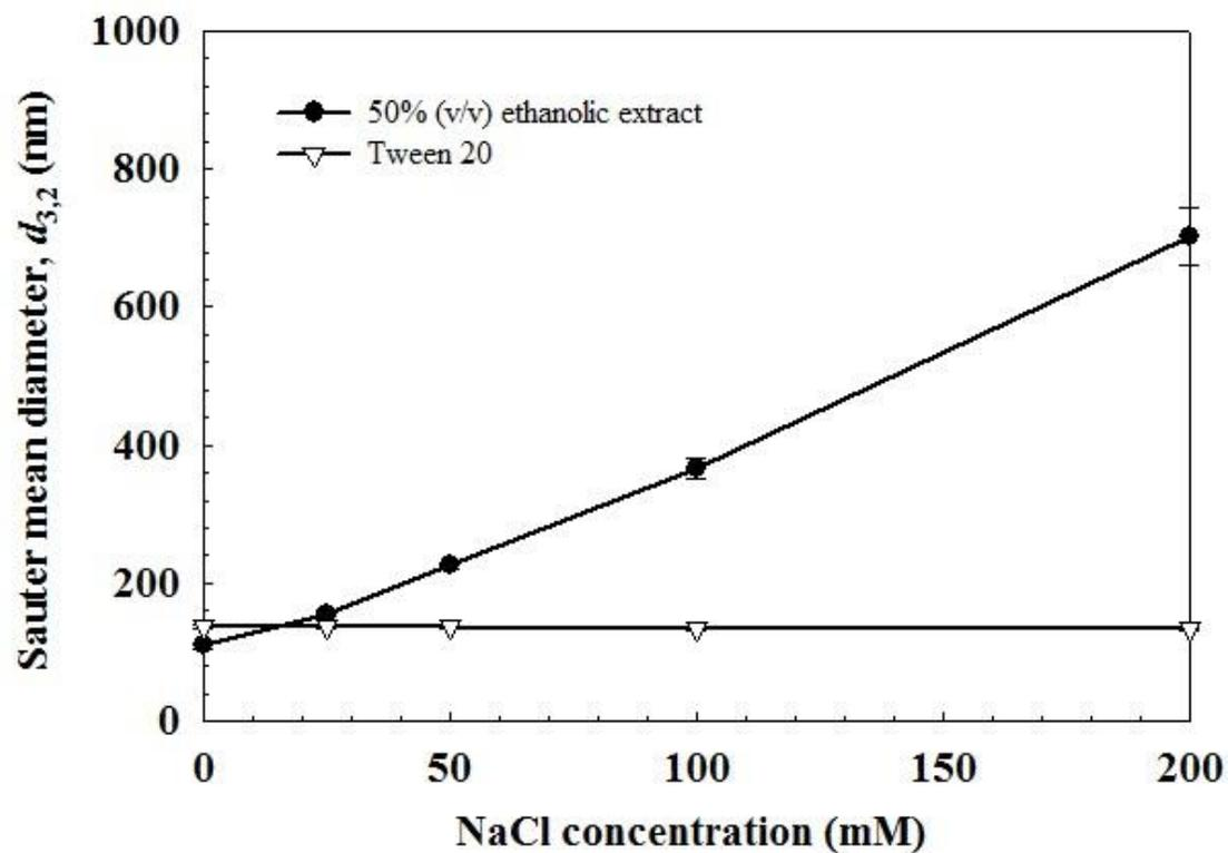
Figure 8. Effect of ionic strength on the  $d_{3,2}$  of 10% (w/w) soybean O/W emulsions containing 2% (w/w) of Tween 20 or 50% (v/v) ethanolic extract.
