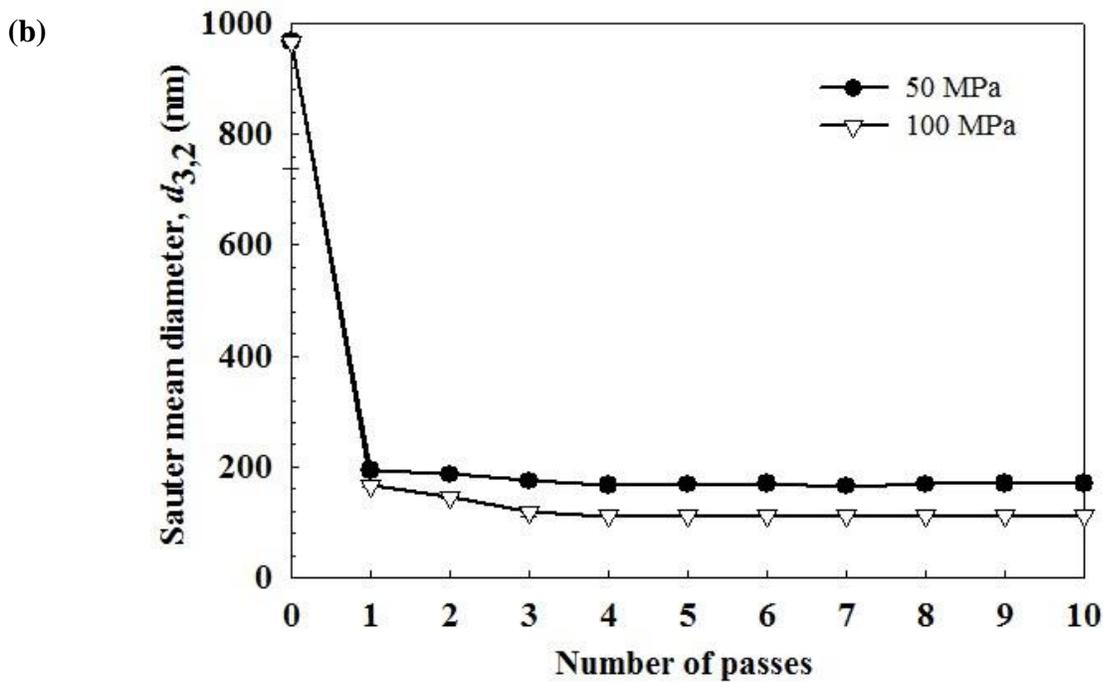
Figure 4. Effect of (a) homogenization pressure and (b) number of passes through the high-pressure homogenizer (100 MPa) on the Sauter mean diameter ( $d_{3,2}$ ) of 10% (w/w) soybean O/W emulsions containing 2% (w/w) of 50% (v/v) ethanolic extract.
