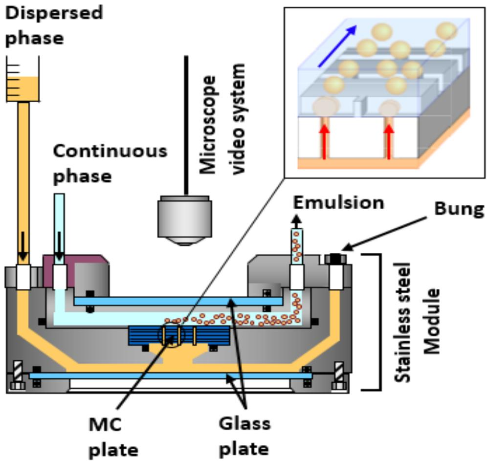
Figure 13. Schematic representation of MCE setup used in this study.
