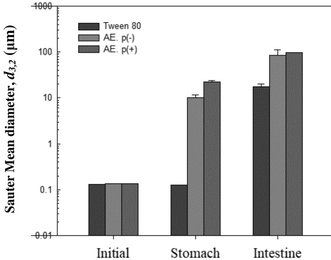
Figure 9. Effect of simulated gastrointestinal conditions on the Sauter mean diameter ( $d_{3,2}$ ) of emulsions prepared using argan extract. AE. p(+) refers to argan extract-based emulsions digested in the presence of pepsin. AE. p(-) refers to argan extract-based emulsions digested in the absence of pepsin.
