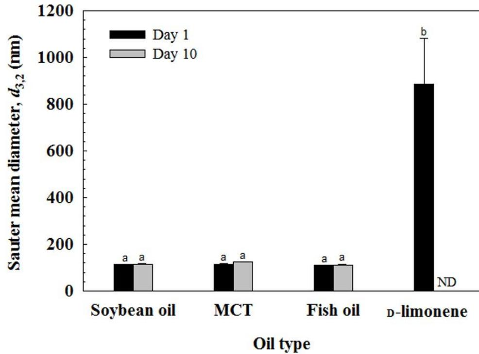
Figure 6. Effect of oil type on the Sauter mean diameter ( $d_{3,2}$ ) of 10% (w/w) O/W emulsions containing 2% (w/w) of 50% (v/v) ethanolic extract. ND: Not detected.
