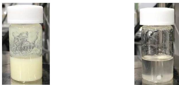
Figure 2.4.5. Diphenylamine + KOtBu(left) and Diphenylamine + NaOtBu(right)
