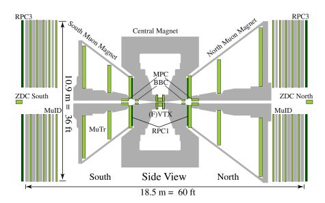
FIG. 2. A side view of the PHENIX detector, concentrating on the muon arm instrumentation. Of primary importance to this analysis are the BBC, FVTX, RPC, MuTr, and MuID. Please see text for descriptions of these subsystems and how they were used.
