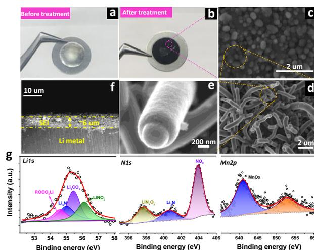
**Figure 1.** Pre-treated method, SEM imaging and XPS spectra of SEI. (a) Li metal on stainless steel without pre-treatment. (b) Li metal immersion in  $\text{Mn}(\text{NO}_3)_2$  additive electrolyte within 1 min. (c) SEM imaging of SEI in (b). (d) Nanotubes morphology of the spherical shape in (c). (e) The zoom in figure of nanotube based on figure (d). (f) The cross-section of SEI in (b). (g) XPS spectra of SEI in (b) for the elements Li1s, N1s, and Mn2p.
