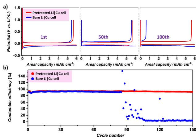
**Figure 2.** The contrast of Li stripping/plating performance of pretreated-Li|Cu cell and bare Li|Cu cell. (a) Voltage profiles of the Li stripping/plating on Cu substrate in the electrolyte of  $1.0 \text{ M LiPF}_6$  in EC/DEC for the 1st, 50th and 100th cycle, respectively. (b) Cycling performance of pretreated-Li|Cu cell and bare Li|Cu cell. Both in (a) and (b), the current density is  $3 \text{ mA cm}^{-2}$  and areal capacity is  $6 \text{ mAh cm}^{-2}$ .
