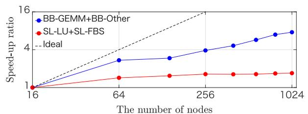
Fig. 2. Scalability of Block BiCGrQ and ScaLAPACK's PZGETRF and PZGETRS.
