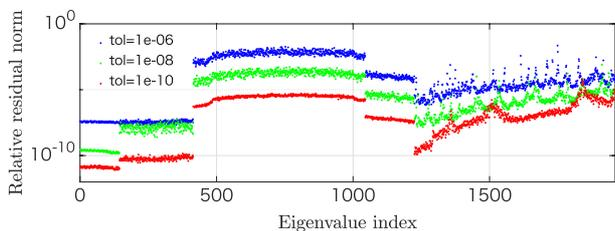
Fig. 4. Relative residual norms of computed eigenpairs by SSM-BB with 3 tolerances.
