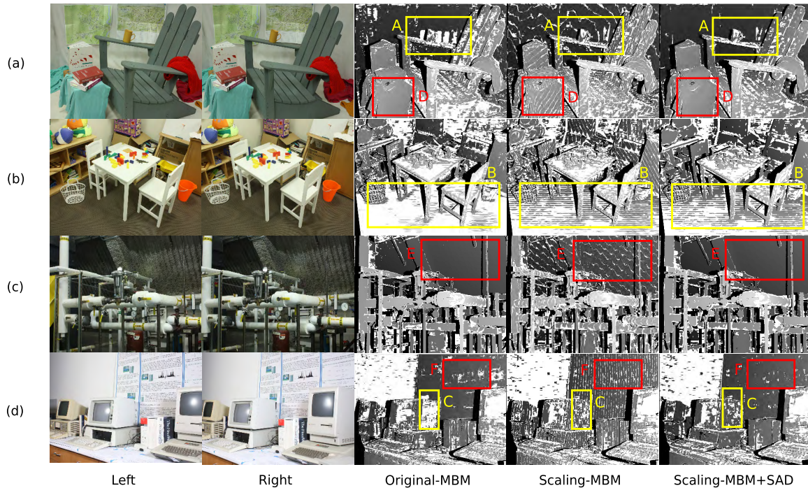
FIGURE 13. Matching Result. (a) Adirondack (b) Playtable (c) Pipes (d) Vintage. A: Repetitive patterns. B: Perspective distortions & Uniform regions. C: Uniform regions. D,E,F: Gradient regions.
