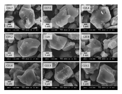
Fig. 4 SEM micrographs of the synthesized Li<sub>2</sub>CoTi<sub>3</sub>O<sub>8</sub> powders (heat-treated at 1100 °C in air for 2 h).
