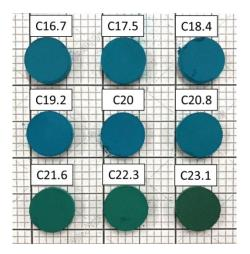
**Fig. 2** Appearance of the synthesized Li<sub>2</sub>CoTi<sub>3</sub>O<sub>8</sub> powders with different CoO compositions (heat-treated at 1100 °C in air for 2 h, and uniaxially pelletized).
