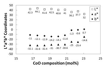
Fig. 5 CIE-L\*a\*b\* color coordinates of the synthesized Li<sub>2</sub>CoTi<sub>3</sub>O<sub>8</sub> powders with different CoO compositions (heat-treated at 1100 °C in air for 2 h, and uniaxially pelletized as shown in Fig. 2).
