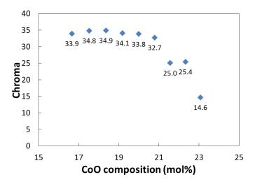
**Fig. 6** Chroma *C*\* of the synthesized Li<sub>2</sub>CoTi<sub>3</sub>O<sub>8</sub> powders with different CoO compositions (heat-treated at 1100 °C in air for 2 h, and uniaxially pelletized as shown in Fig. 2).
