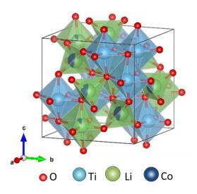
Fig. 1 Crystal structure of Li<sub>2</sub>CoTi<sub>3</sub>O<sub>8</sub> drawn with a reported data by Kawai et al [12].
