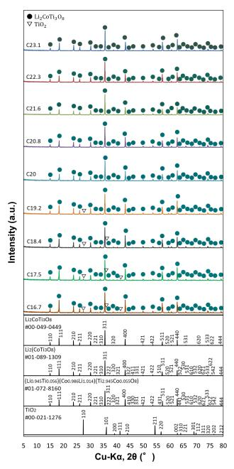
Fig. 3 XRD patterns of the synthesized Li<sub>2</sub>CoTi<sub>3</sub>O<sub>8</sub> powders (heat-treated at 1100 °C in air for 2 h). Reported XRD patterns for Li<sub>2</sub>CoTi<sub>3</sub>O<sub>8</sub> and TiO<sub>2</sub> rutile are also shown.
