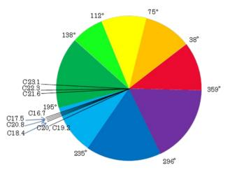
Fig. 7 Hue angle *h* of the synthesized  $Li_2CoTi_3O_8$  powders with different CoO compositions (heat-treated at 1100 °C in air for 2 h, and uniaxially pelletized as shown in Fig. 2), displayed on a 2-D simplified  $L^*a^*b^*$  color space diagram cut in the horizontal direction. Dichromatic color nature, *i.e.*, cyan and green, was confirmed.
