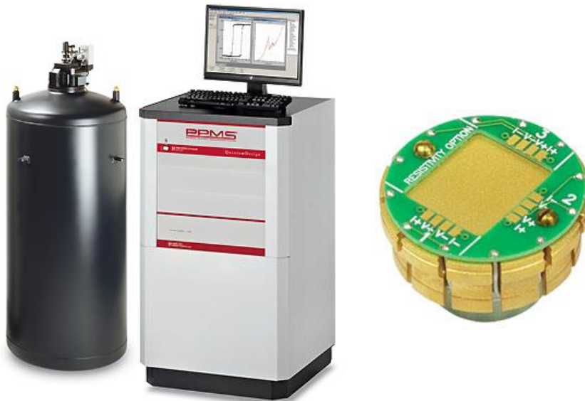
Figure 2. 9 shows physical property measurement system (PPMS) and AC Transport Puck used as sample holder on the right side Ref [137]
