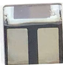
Fig. 2.6 Appearance of the perovskite solar cell. The cell size is 12.5 \times 12.5 \text{ mm}^2 .
